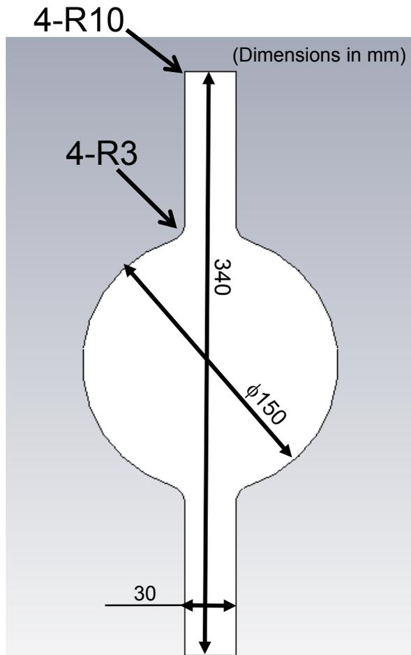
(Cross-section perpendicular to the beam axis)
