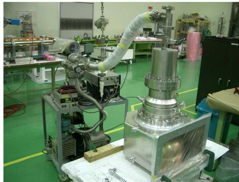
➔ Tested in the upgrade coupler test stand
