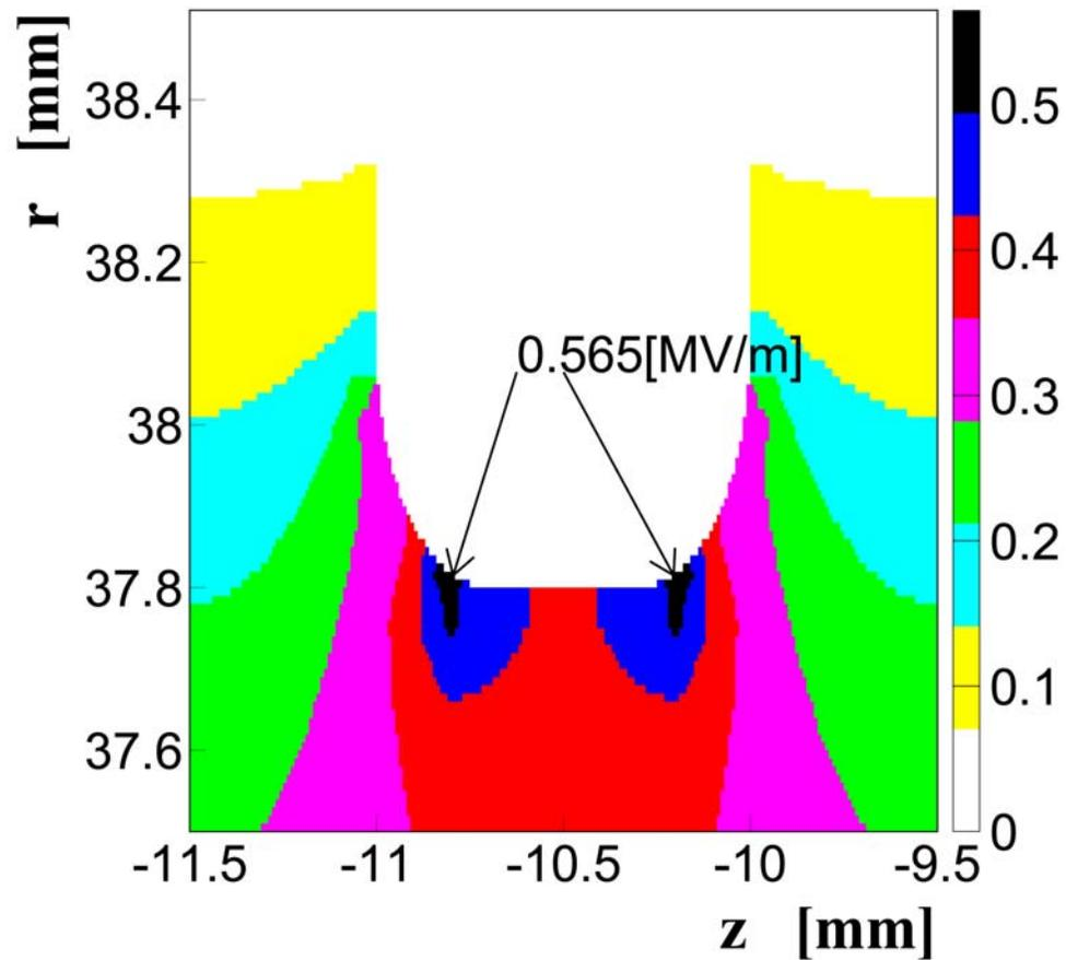
The max. 0.565[MV/m] is lower than that on the inner conductor of the coaxial line with no groove (=0.717[MV/m]).
