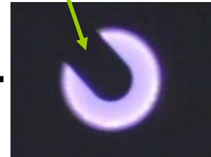
Example of the TV-camera snapshots of the *multipactoring* in the **coaxial line**
