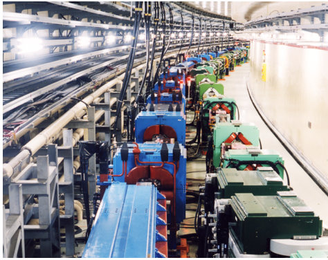
Figure 4: KEKB arc section. Two rings (HER and LER) were placed horizontally, thanks to wide TRISTAN tunnel.
