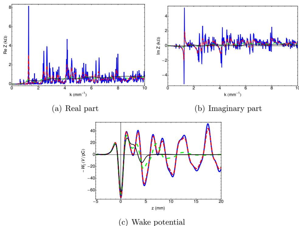
**Figure 2.15:** CSR impedance and wake potential of the arc section in the SuperKEKB positron damping ring. The impedances and wake potentials have been normalized by the number of cells. The gaussian bunch length  $\sigma_z = 0.5$  mm with bunch head to the left side. Blue solid line: 16 cells; red dashed line: 6 cells; Green dashed line: 1 cell; Black solid line: single-bend model.
