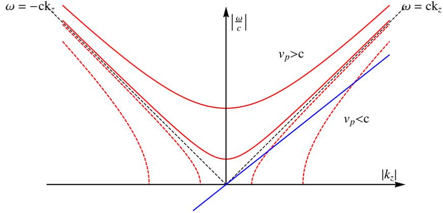
**Figure 3.4:** Dispersion relation for the waves excited by a point charge moving along a perfectly conducting waveguide with  $v < c$ . The solid blue line denotes the beam mode.
