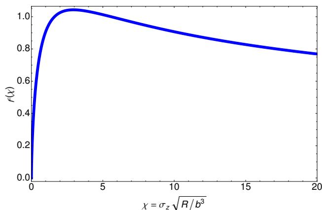
**Figure 4.1:** Ratio of the thresholds of coasting beam model to the bunched beam model, as a function of shielding parameter.
