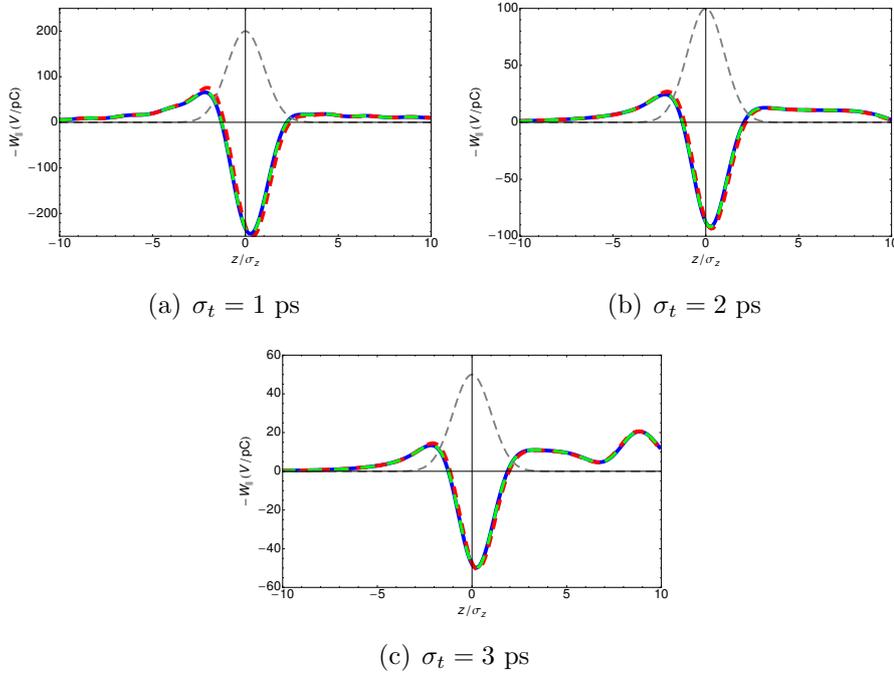
**Figure 2.17:** CSR wake potentials for a single bend in the cERL return loop with Gaussian bunch lengths of  $\sigma_t = 1, 2, 3$  ps. The drift CSR is taken into account. Blue solid lines:  $\gamma = \infty$ ; red dashed lines:  $\gamma = 68.5$  ( $E = 35$  MeV); green dashed lines:  $\gamma = 244.6$  ( $E = 125$  MeV); gray dashed lines: Gaussian bunch profile.
