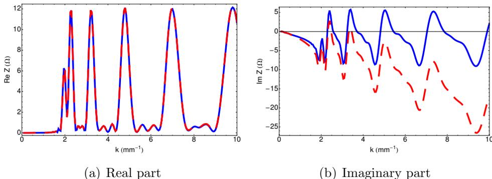
**Figure 3.9:** CWR impedance of a wiggler with high order modes considered. The blue solid represents the result with only low order modes considered; the red dashed line stands for the result with high order modes also taken into account.
