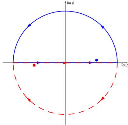
**Figure 3.3:** Contour for the complex integration over  $\beta$ . The blue solid line is for  $z - z' > 0$ ; the red dashed line is for  $z - z' < 0$ . The blue and red dots represent the singular points in the upper and lower plane, respectively.
