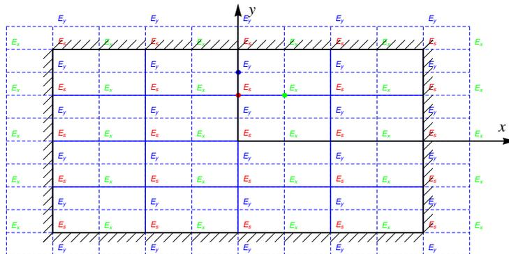
**Figure 2.3:** Staggered grid definition with ghost points outside the boundary of the chamber. The positions of various field components are shown. Constant spacing in the  $x$  and  $y$  directions is assumed.
