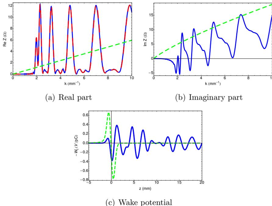
**Figure 2.22:** CSR impedance and wake potential of a wiggler. The blue lines are numerical results. The dashed red line and dashed green lines are given by Eq. (2.90) and Eq. (2.93), respectively. The gaussian bunch length  $\sigma_z = 0.5$  mm with bunch head to the left side.
