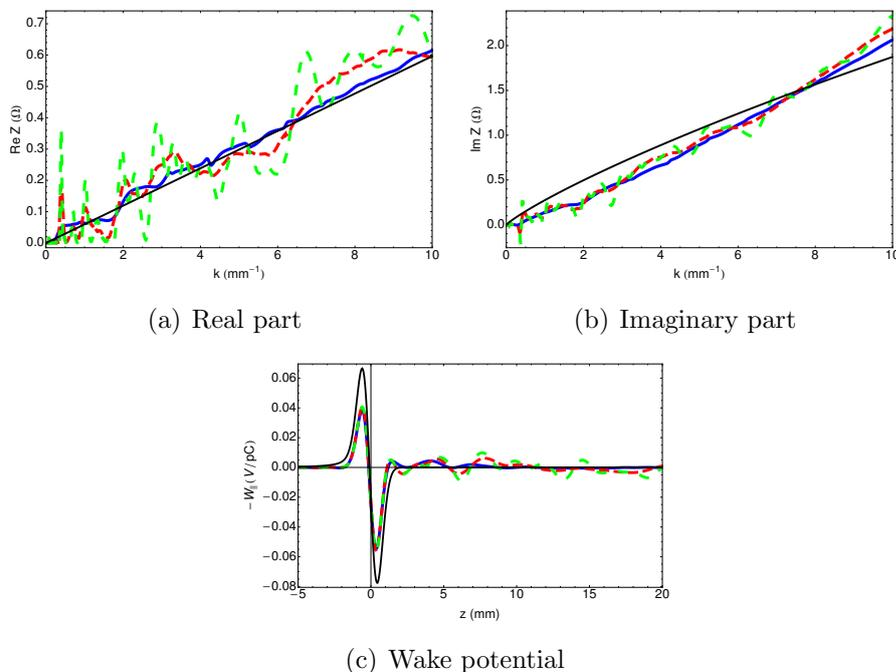
**Figure 2.24:** CSR impedance and wake potential of a wiggler with the total length varied by setting  $N_u = 1, 4, 8$ . The impedances and wake potentials have been normalized by the number of period for convenience of comparison. The gaussian bunch length  $\sigma_z = 0.5$  mm with bunch head to the left side. Blue solid lines:  $N_u = 1$ ; red dashed lines:  $N_u = 4$ ; green dashed lines:  $N_u = 8$ ; black solid lines: free-space model.
