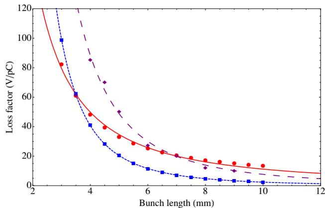
**Figure 4.5:** Comparison of calculated and measured loss factor as a function of bunch length for KEKB LER. Purple dots: measured data; red dots: calculated from numerical wakes; blue dots: calculated from resonator model. The lines are fitted curves as described in the text.
