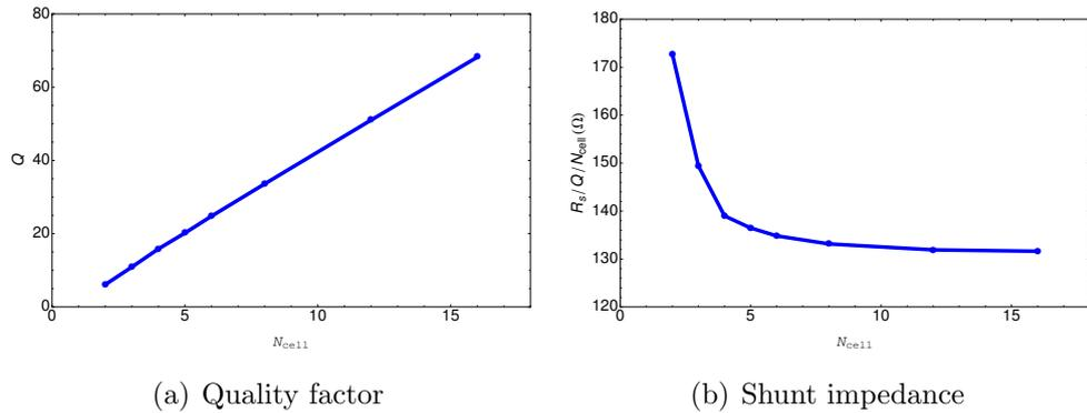
**Figure 4.9:** Quality factor and shunt impedance as a function of number of cells at the resonant peak of  $k_r = 1.264 \text{ mm}^{-1}$ . CSR impedances are calculated using different number of cells in one arc section of SuperKEKB positron damping ring dipole magnets. The shunt impedances have been normalized by the number of cells and quality factor.
