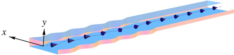
**Figure 2.2:** The geometry of the curved chamber for a wiggler. An infinitely long straight chamber is connected after the exit of the curved chamber. The beam moves along the curved line with arrows. The origin of the coordinate system coincides with the beam orbit.
