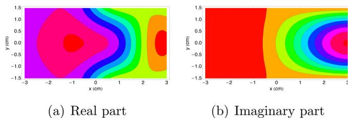
**Figure 2.8:** Contour plots for the profiles of the radiation field  $E_x^r$  at the exit of the curved chamber with  $k = 1230 \text{ m}^{-1}$  and  $L_b = 8 \text{ m}$ . The outer wall of the chamber is to the right side.
