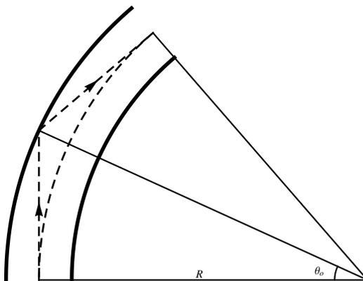
**Figure 2.7:** CSR reflected by the outer wall of the beam pipe. The beam starts to radiate fields at the entrance of the curved chamber. The dashed curve without arrows on it denotes the beam orbit. The arrowed dashed lines represent the direction of the radiation fields.
