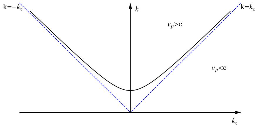
**Figure 3.1:** Parabolic dispersion relation, typical of waves propagating in a waveguide. The cutoff frequency is reached for  $k_z = 0$ . The dashed lines split the plane into fast- and slow-wave regions.
