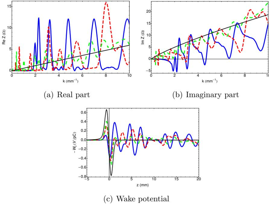
**Figure 2.23:** CSR impedance and wake potential of a wiggler with  $b = 2, 5, 10$  cm. The gaussian bunch length  $\sigma_z = 0.5$  mm with bunch head to the left side. Blue solid lines:  $b = 2$  cm; red dashed lines:  $b = 5$  cm; green dashed lines:  $b = 10$  cm; black solid lines: free-space model.
