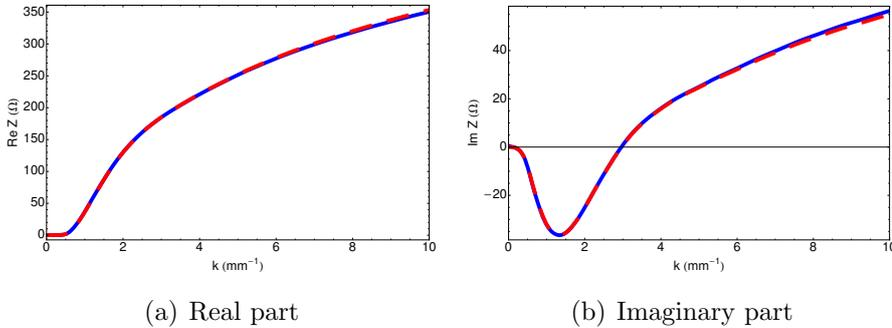
**Figure 2.5:** CSR impedance for a single bending magnet with  $R = 1$  m and  $L_b = 0.2$  m. The dimensions of the chamber cross-section are  $a = 6$  cm, and  $b = 2$  cm. The blue and dashed red lines are given by Stupakov's code and our code, respectively.
