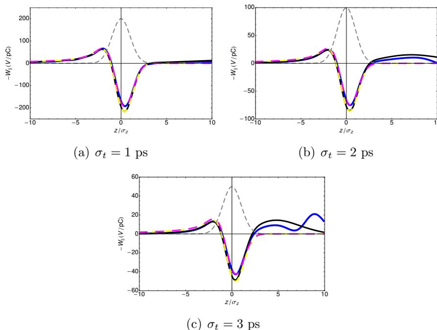
**Figure 2.18:** CSR wake potentials for a single bend in the cERL return loop with Gaussian bunch lengths of  $\sigma_t = 1, 2, 3$  ps and  $\gamma = \infty$ . The drift CSR is not taken into account. Blue solid lines: by CSRZ; magenta dashed lines: 1D model; black solid lines: steady-state parallel plates model; yellow dashed lines: steady-state free space model; gray dashed lines: Gaussian bunch profile.
