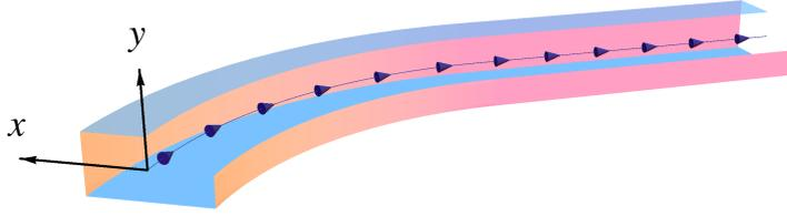
**Figure 2.1:** The geometry of the curved chamber for a single bending magnet. An infinitely long straight chamber is connected after the exit of the curved chamber. The beam moves along the curved line with arrows. The origin of the coordinate system coincides with the beam orbit.
