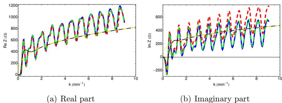
**Figure 2.16:** CSR impedance for a single bend in the cERL return loop. The CSR in the drift chamber after the exit of the bend is taken into account. Blue solid lines:  $\gamma = \infty$ ; red dashed lines:  $\gamma = 68.5$  ( $E = 35$  MeV); green dashed lines:  $\gamma = 244.6$  ( $E = 125$  MeV); black solid lines: steady-state parallel plates model; yellow dashed lines: steady-state free space model.
