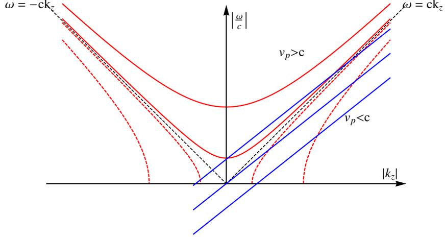
**Figure 3.7:** Dispersion relation for the waves excited by a point charge moving along a perfectly conducting waveguide sandwiched by a wiggler. The solid blue line denotes the beam mode.
