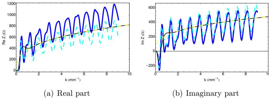
**Figure 2.19:** CSR impedance for a single bend in the cERL return loop with  $\gamma = \infty$ . Blue solid lines: with drift CSR considered; cyan dashed lines: with drift CSR neglected; black solid lines: steady-state parallel plates model; yellow dashed lines: steady-state free space model.
