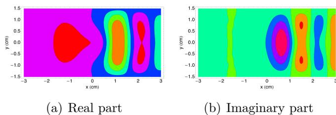
**Figure 2.9:** Contour plots for the profiles of the radiation field  $E_x^r$  at the exit of the curved chamber with  $k = 4930 \text{ m}^{-1}$  and  $L_b = 8 \text{ m}$ . The outer wall of the chamber is to the right side.
