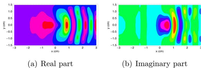
**Figure 2.10:** Contour plots for the profiles of the radiation field  $E_x^r$  at the exit of the curved chamber with  $k = 9100 \text{ m}^{-1}$  and  $L_b = 8 \text{ m}$ . The outer wall of the chamber is to the right side.
