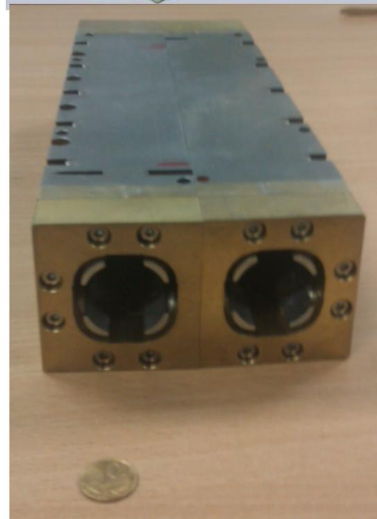
Saddle-shaped coils, complicated in production, the first coil failed. New winding device is in development.
