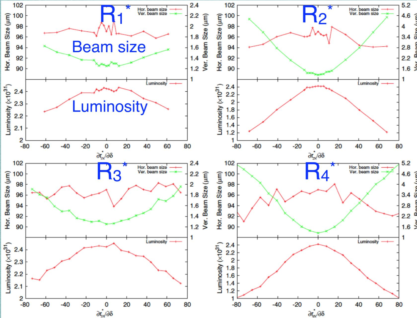
FIG. 8. (Color) Scan of first-order chromaticity of X-Y couplings at the IP.
