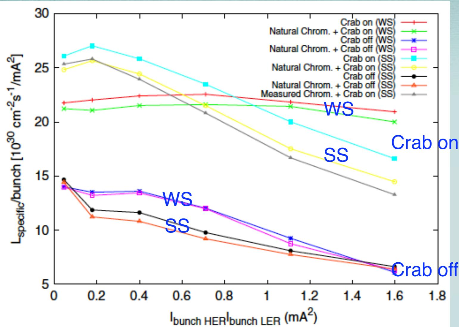
FIG. 5. (Color) Specific luminosity as a function of current product for KEKB. The natural chrom. and measured chrom. indicate natural chromaticity and measured chromaticity calculated from ideal optics and measurement data at KEKB HER, respectively. The WS and SS represent weak-strong and strong-strong simulations, respectively.
