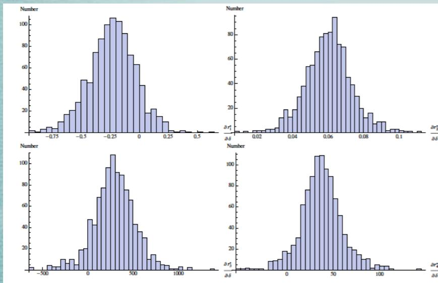
Figure 3: Distributions of the chromatic X-Y couplings with 1000 error seeds for the SuperKEKB LER.
