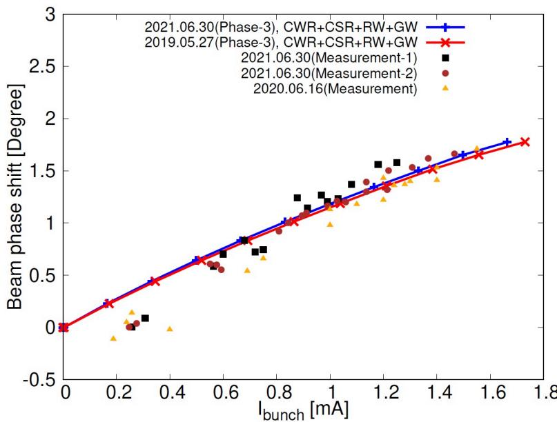
Comparison of center-of-mass shift with synch. Phase shift, the agreement is not good at low bunch currents.
