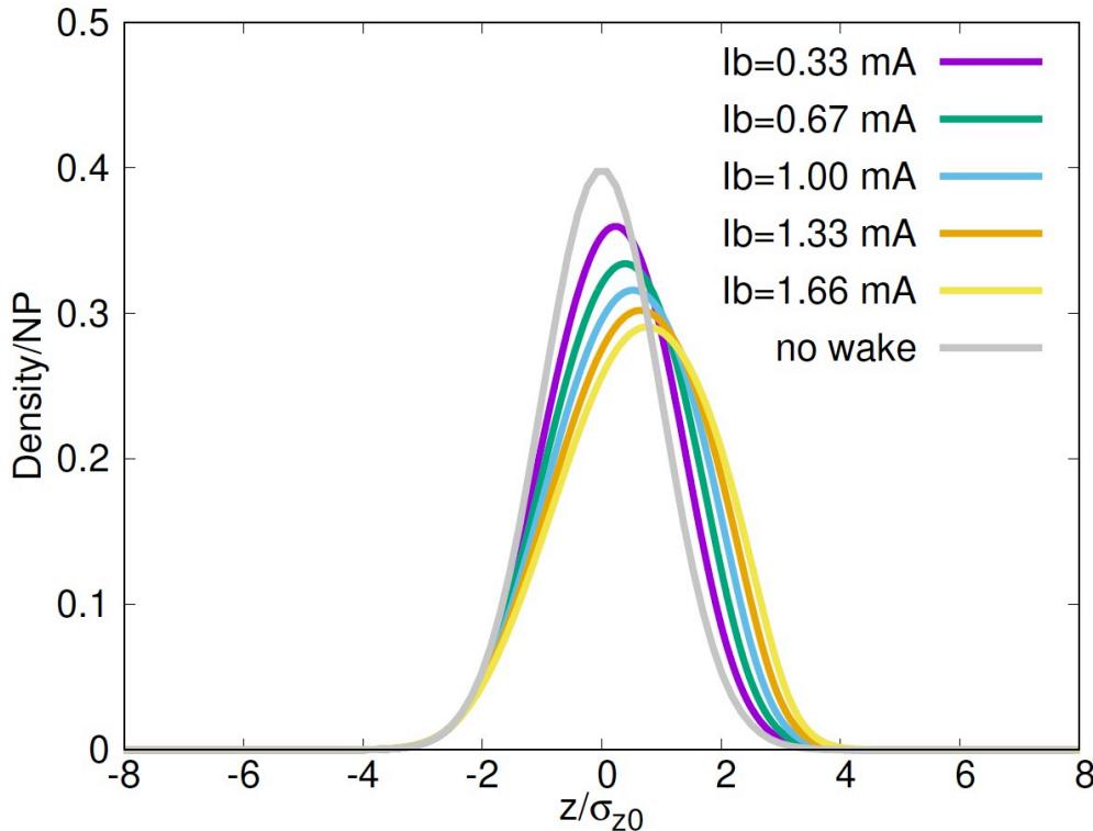
Simulated bunch profiles have tilt and shift in center-of-mass.
