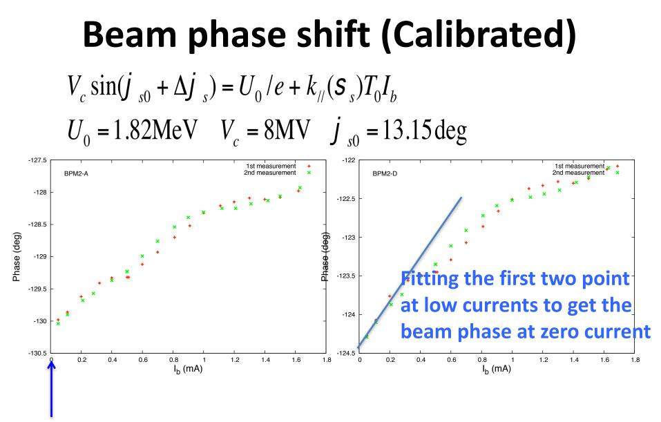
Beam phase at zero current is important...
