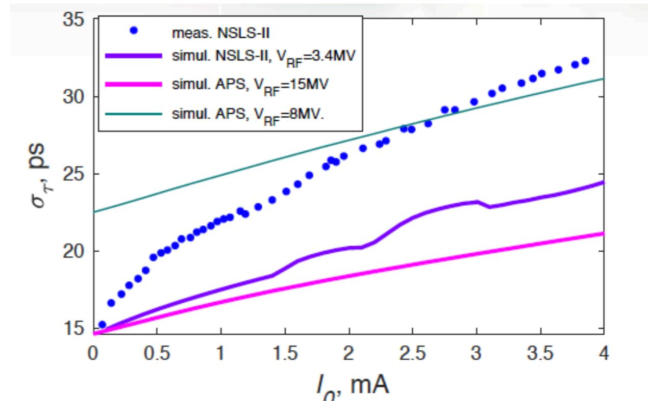
Streak camera measurements of the bunch length as a function of single-bunch current  $\sigma_\tau(I_0)$  vs VFP particle tracking simulations at  $V_{RF} = 3MV$
