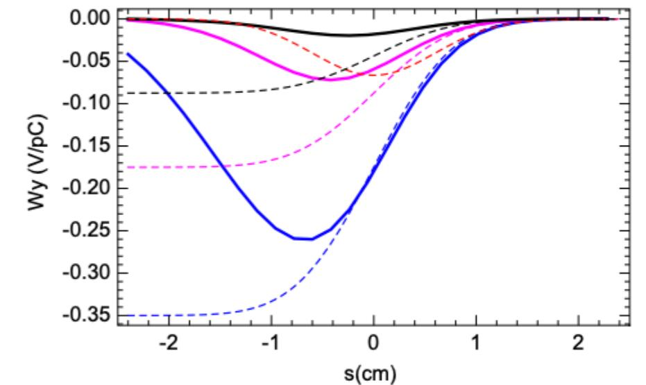
Fig. 3. Wakefield of a bunch with  $\sigma_z = 6$  mm for three values of the protrusion depth  $h$ : 1 cm (blue), 0.5 cm (magenta) and 0.25 cm (black). The dashed lines of the same color show the corresponding wakes computed with the optical model. The red dashed line shows the profile of the beam. (For interpretation of the references to color in this figure caption, the reader is referred to the web version of this article.)
