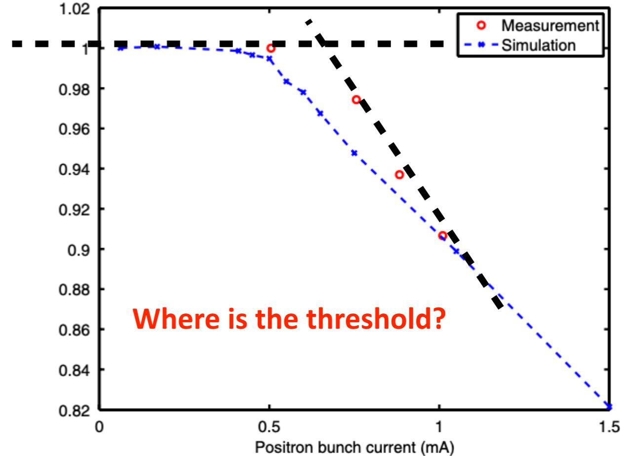
FIG. 6. (Color) Ratio of hadron events to Bhabha was measured as a function of positron bunch current using the Belle detector. The data is normalized to the measured value at 0.5 mA. The result of simulation is plotted according to Eq. (18) and the energy spreads at zero currents are used for the normalization.
