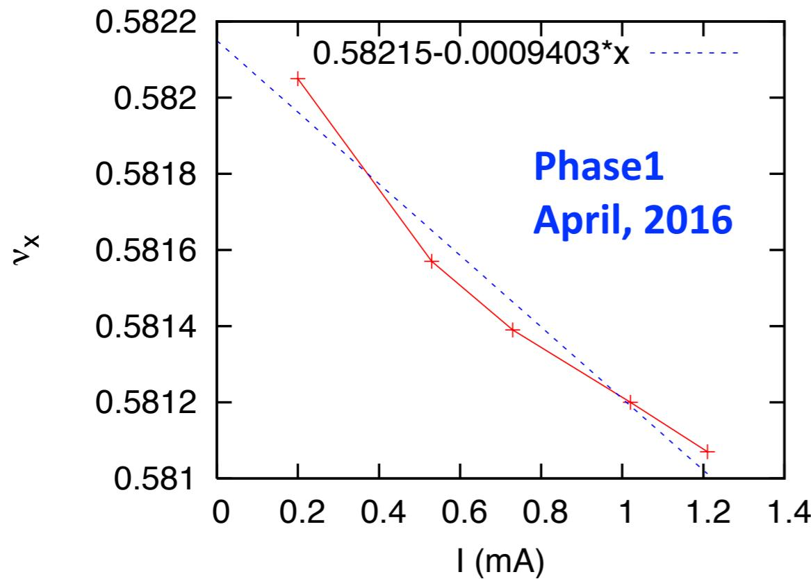
$$iZ_{\text{eff}}^X = 37 \text{ k}\Omega/\text{m}$$
