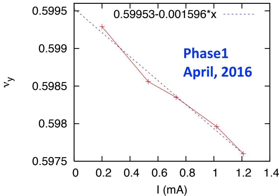
$$iZ_{\text{eff}}^Y = 106 \text{ k}\Omega/\text{m}$$
