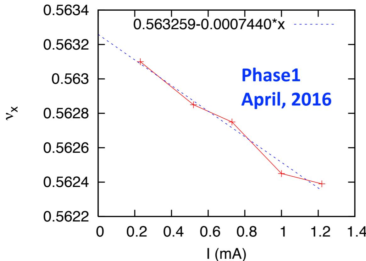
$$iZ_{\text{eff}}^X = 71 \text{ k}\Omega/\text{m}$$
