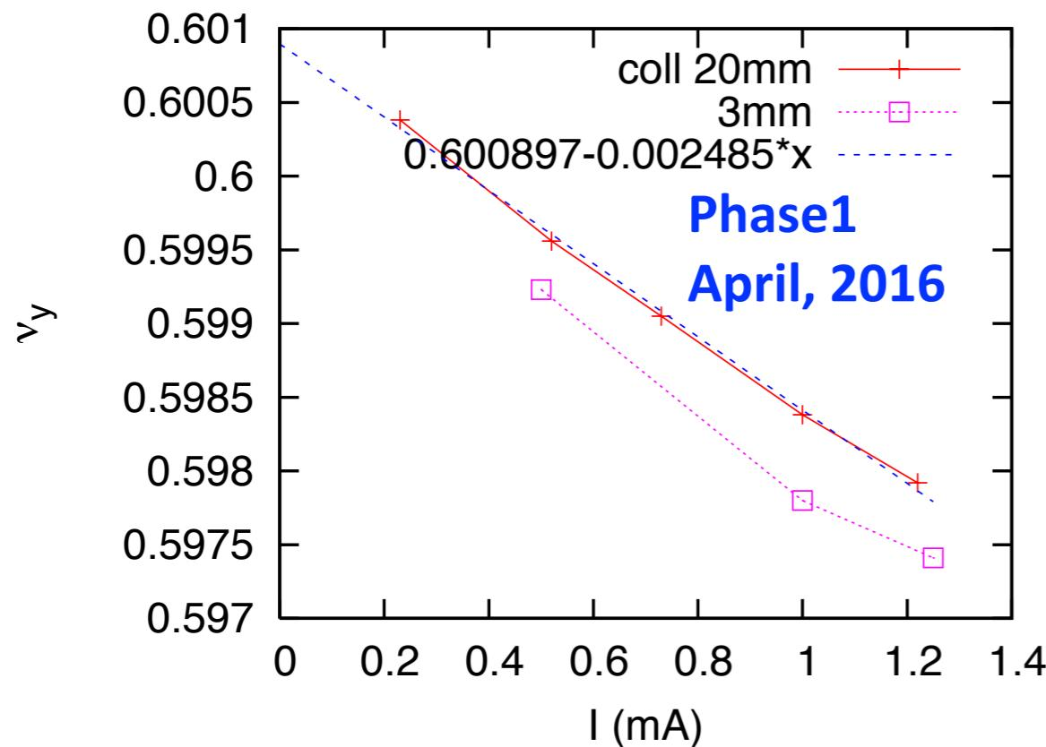
$$iZ_{\text{eff}}^Y = 247 \text{ k}\Omega/\text{m}$$
