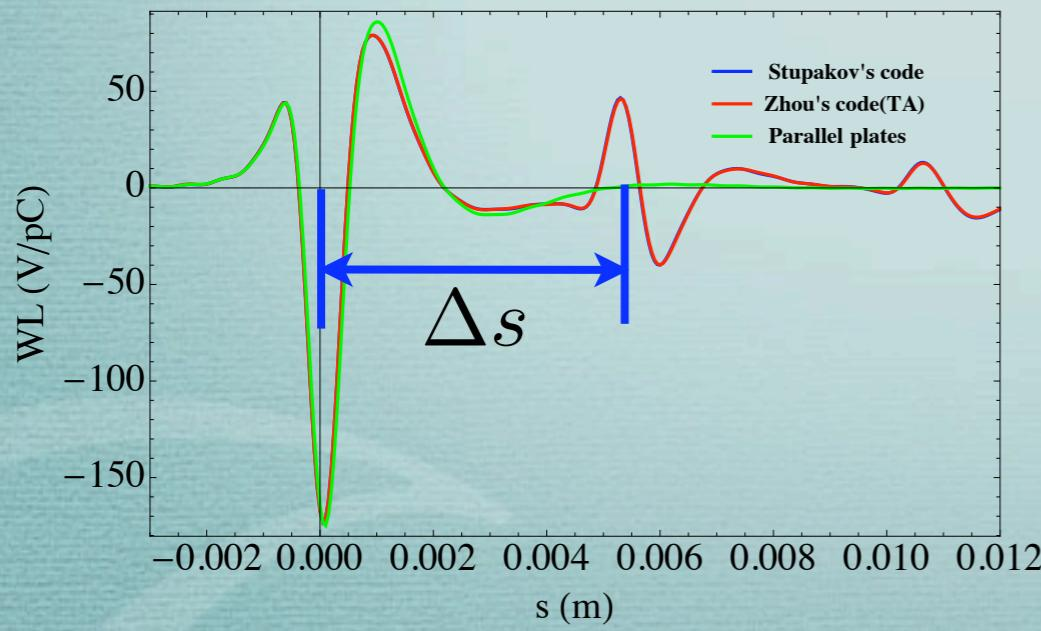
**Fluctuation in impedance is due to reflections of side walls (Oide)**
