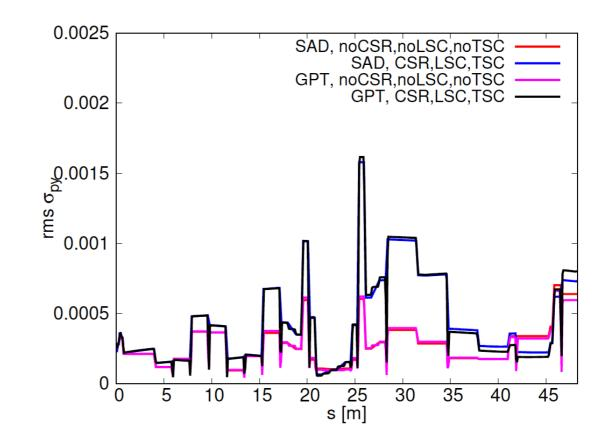
rms vertical beam size and momentum spread with average LSC model
