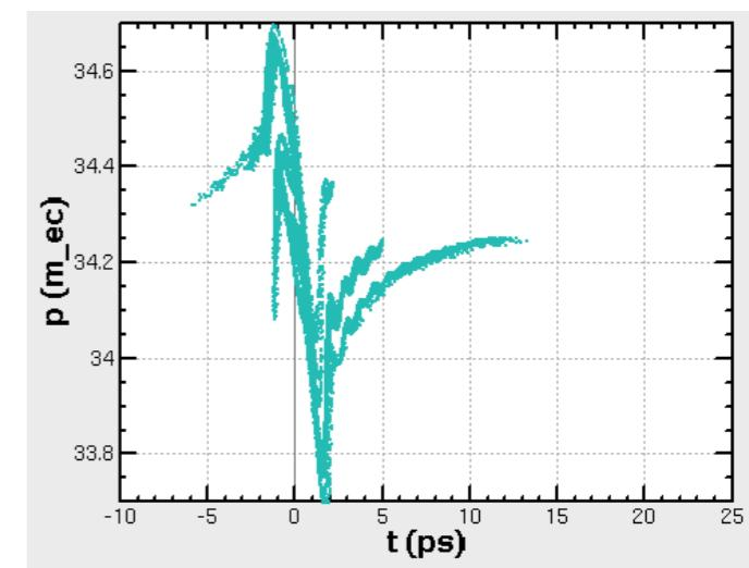
SAD simulation: The SC forces are calculated using Gaussian fitted  $\sigma_x$  and  $\sigma_y$ , and arbitrary density (histogram) in  $z$  direction.
