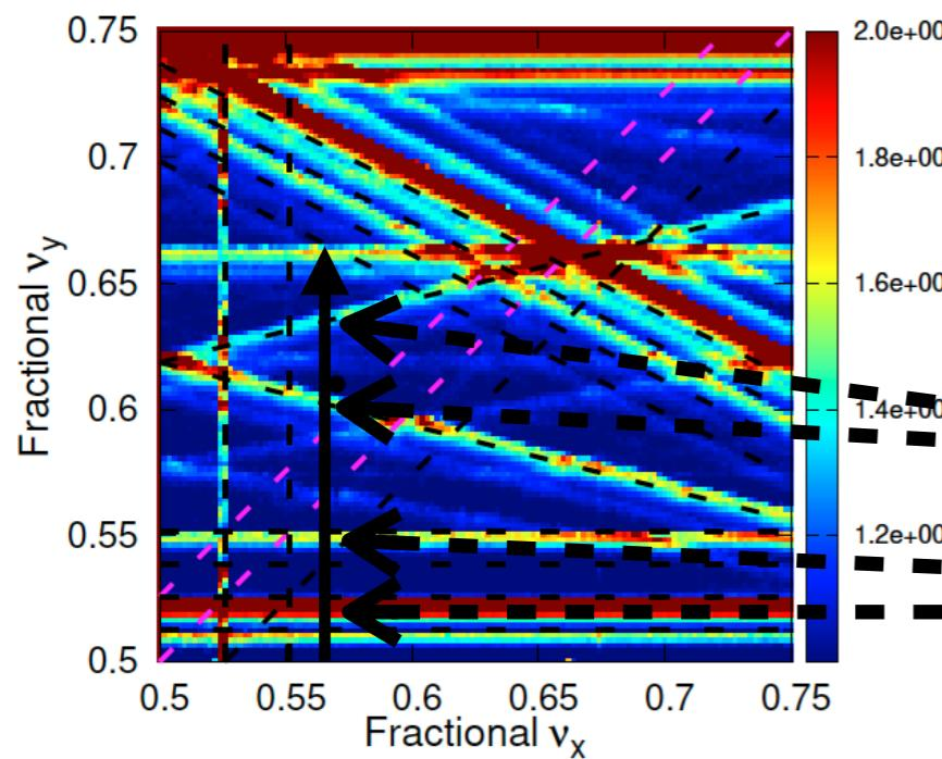
Beam sizes for  $v_{s+}=.0225$ ,  $v_{s-}=.0258$
