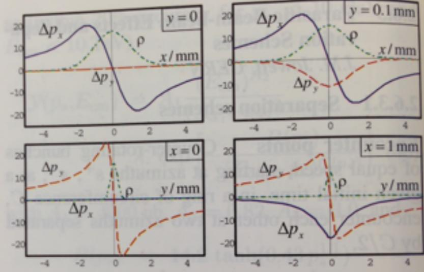
Figure 4: Beam-beam kicks in  $\mu\text{rad}$  felt by a 1 GeV,  $Z = -1$ , particle (e.g., electron) as a function of horizontal (left) and vertical (right) separations around a bunch with  $N = 10^{10}$ ,  $\sigma_x = 1 \text{ mm}$ ,  $\sigma_y = 0.2 \text{ mm}$  (e.g., positron bunch). In the plots on the left, the other separation is zero, while on the right a non-zero separation is included. Each plot has the same scales and the (scaled) Gaussian charge density is also shown.
