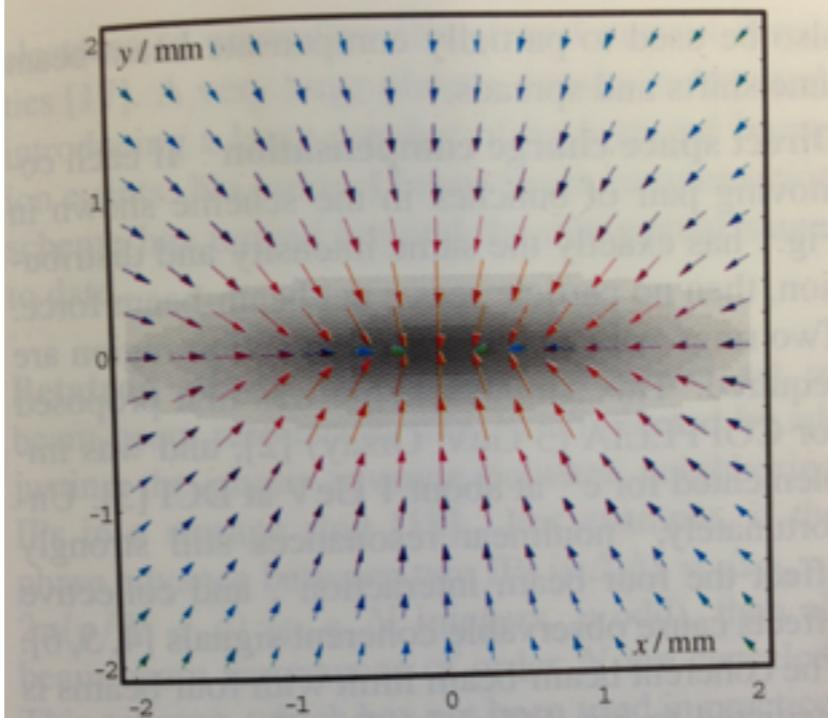
Figure 5: Kick vector field where the length (and color) of the arrows indicates the kick strength. Gray shading indicates the charge density. Same parameters as Fig.4.
