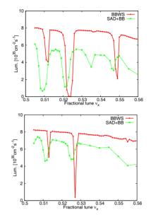
Figure 1: Total luminosity as a function of horizontal tune. Top picture is for LER, and bottom picture is for HER.
