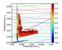
Figure 3: FMA plot for the LER in the plane of betatron tunes.
