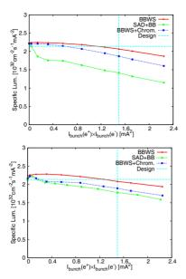
Figure 2: Specific luminosity as a function of bunch current products. Top picture is for LER, and bottom picture is for HER.
