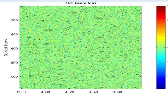
TbT beam loss rate (a.u.) during the last 100 turns by BCM
