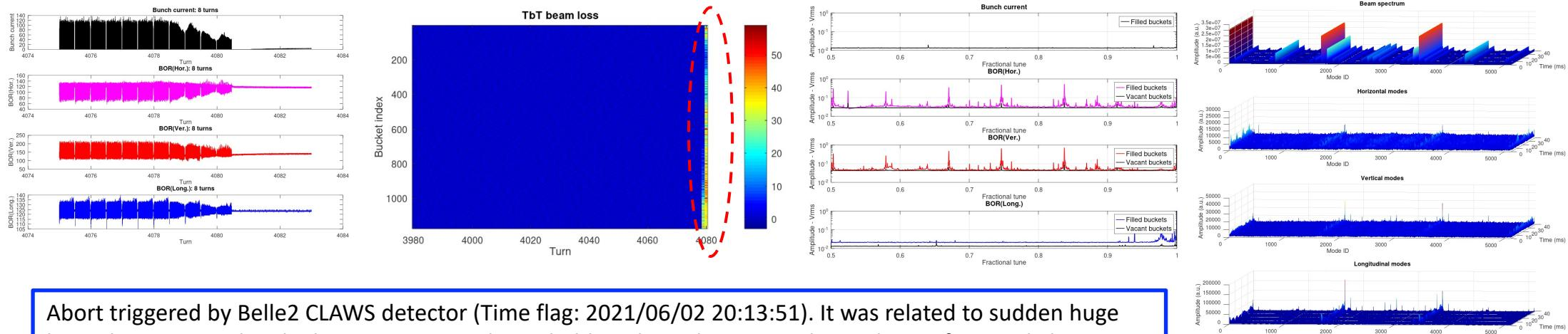
Abort triggered by Belle2 CLAWS detector (Time flag: 2021/06/02 20:13:51). It was related to sudden huge beam loss in LER. The TBT beam spectra and coupled-bunch modes are similar to those of manual abort.
