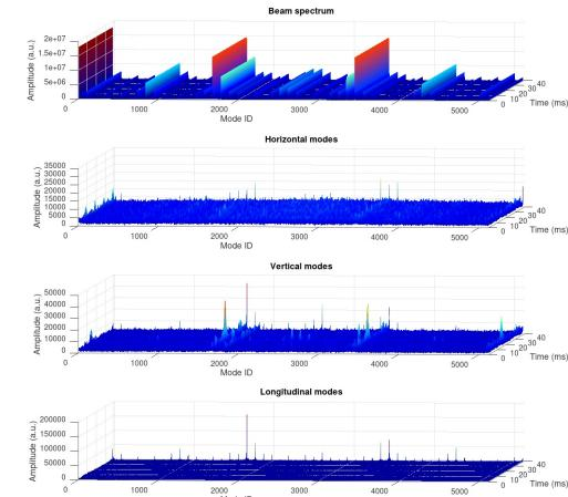
Abort triggered by Belle2 CLAWS detector (Time flag: 2021/06/22 01:22:07). It was related to sudden small beam loss in [HER](#). The TbT beam spectra and coupled-bunch modes are similar to those of manual abort.
