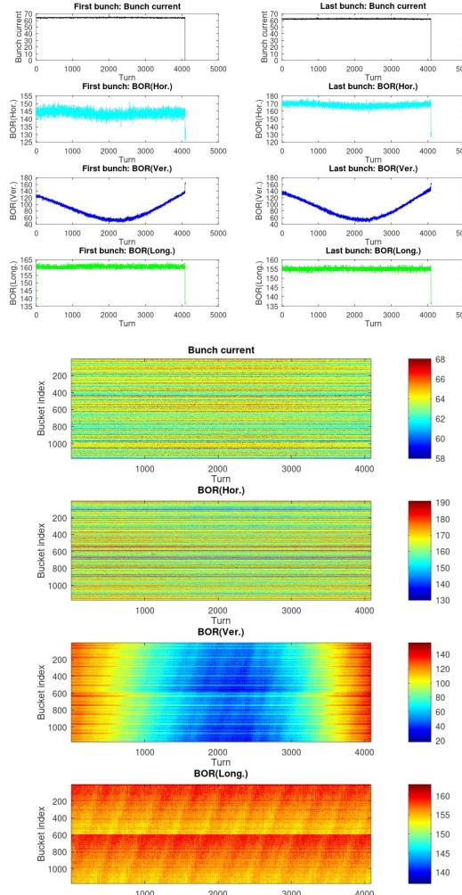
An abort related to earthquake at 23:40 PM, 2021/05/30. The ground motion caused modulation of beam motion in both H/V planes at both HER (LER is similar), resulting in extra Belle2 BG.
