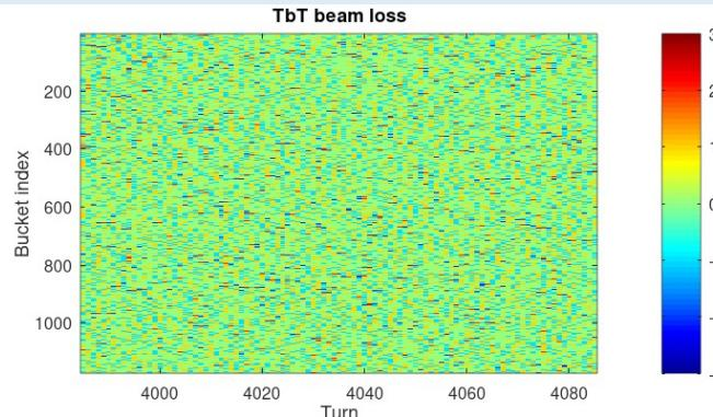
TbT beam loss rate (a.u.) during the last 100 turns by BCM
