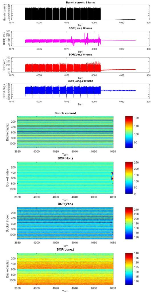
An abort related to LER injection kicker mismatch at 18:39 PM, 2021/06/24. Part of the bunch train in LER was excited in the horizontal direction, resulting in extra Belle2 background which triggered abort.
