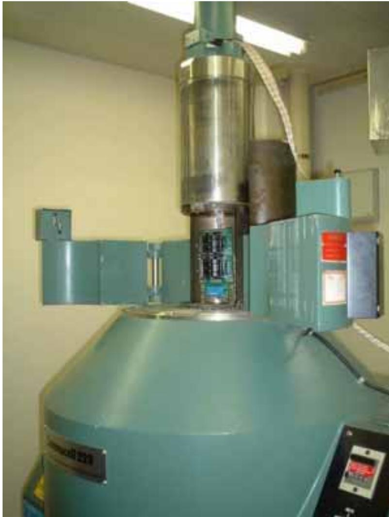
Fig. 1 Photograph of Gamma Cell 220 at Tokyo Metropolitan University. Irradiation chamber is opened and irradiation board of the AMT-2 is located inside. The chamber will go down during irradiation.
