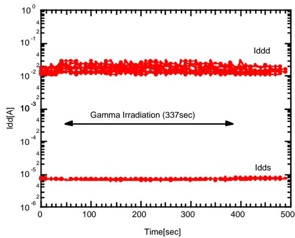
Fig. 4 Variation of static (Idds) and dynamic (Iddd) currents during irradiation. 10 irradiated chip and 1 non\_irradiated chip are plotted
