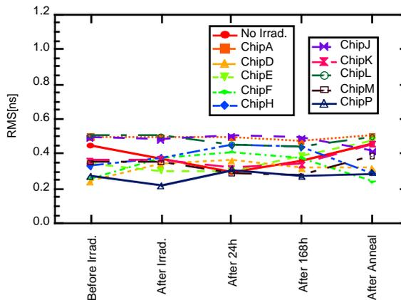
Fig. 6 Time difference measurement of two pulses for 'before irradiation', 'after irradiation', "after 24 hours at room temperature', 'after 168 hours at room temperature', and 'after 168 hours at 100 °C' annealing'.
