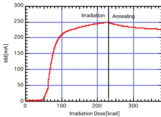
Fig. 5 Leak Current of AMT-2 (measured on Aug. 2001).
