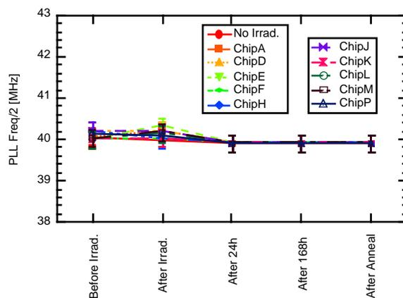
Fig. 7 Frequency variation of PLL clock generated from the PLL.
