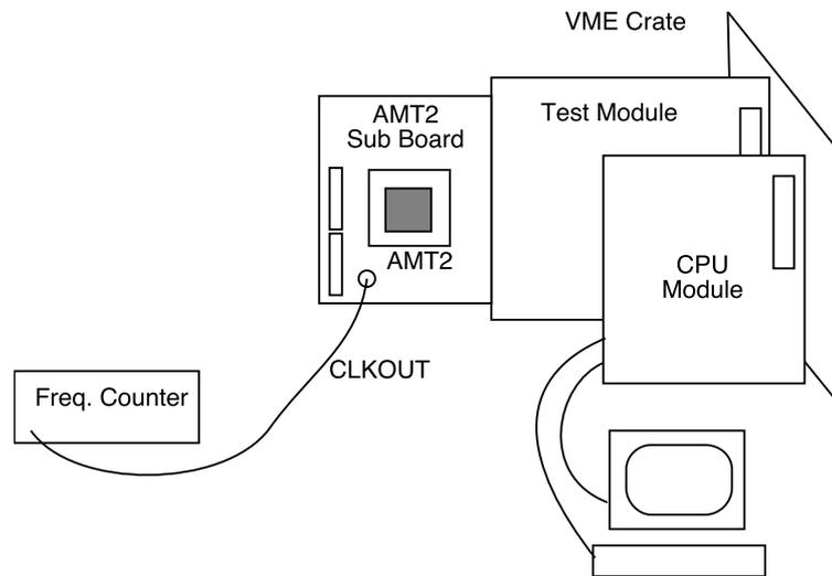
Fig. 3 Measurement setup after Irradiation.
