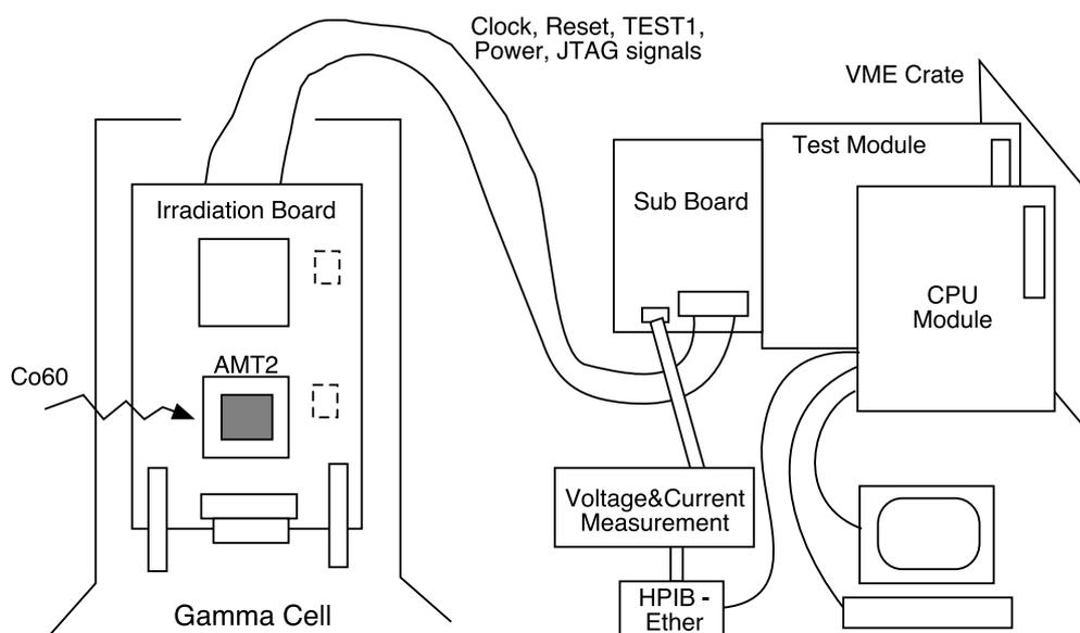
Fig. 2 Irradiation set up with on-line current measurement.
