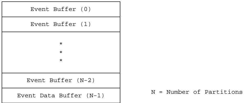
The buffer area is equally divided, so all partitions have the same size. If the data size of an event is larger than the buffer size, an OVR bit in error report word is set and data beyond the buffer size are discarded.
