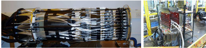
Figure 1: Pictures of the tracker prototype (left) and the cryostat for 2048-channel VLPC (right).
