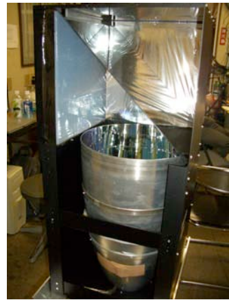
The structure of the prototype of aerogel-based photon counter
