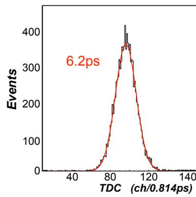
Figure 2: Time difference distribution for 13 mm thick quartz.
