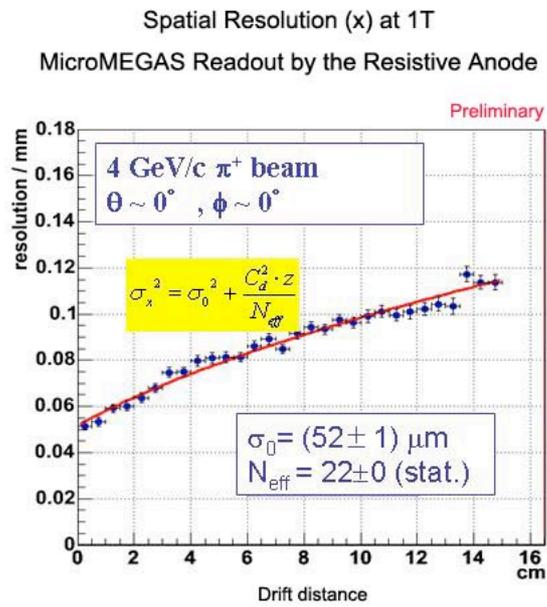
Fig. 5 Spatial resolutions measured for the MicroMEGAS readout by the resistive anode at 1T. The gas mixture was Ar-Isobutene (5%). The width of readout pads was 2 mm. The fitted curb with  $N_{\text{eff}} = 22$  is also shown. The Carleton TPC was used for this measurement.
