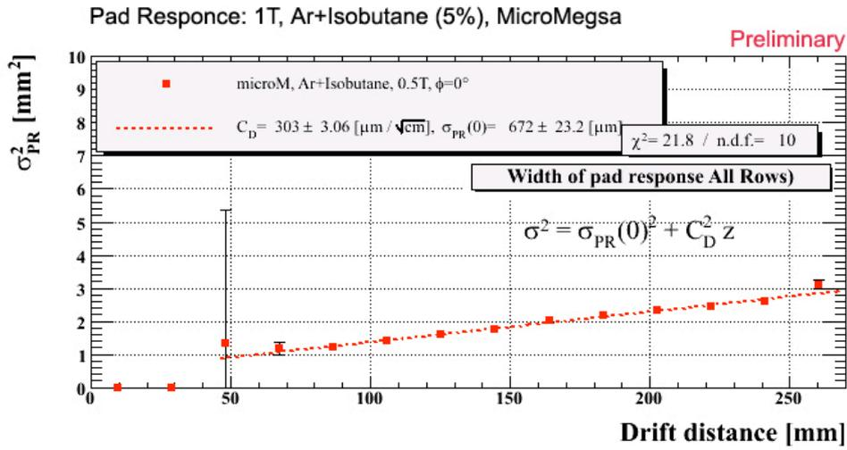
Fig. 1 Measurement of the diffusion constant of Ar-Isobutane (5%) at 0.5T in T572. The pad response is plotted as a function of the drift distance. The MicroMEGAS mounted on the MP TPC was readout by normal pads of 2.1 (2.3) mm wide (pitch).
