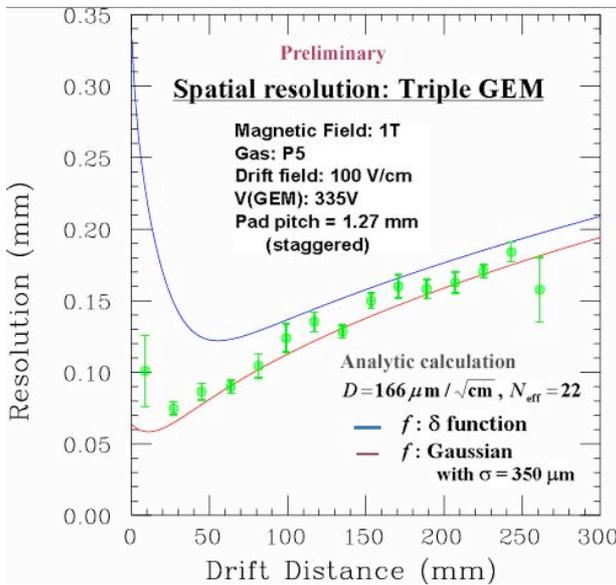
Fig 4 Spatial resolutions measured for the triple GEM at 1T in T783. The gas mixture was P5 and the pad width (pitch) 1.1 (1.3) mm. The curbs are the predictions from the analytic calculation, where  $N_{\text{eff}}$  is assumed to be 22. The width  $\sigma_{\text{PRF}}$  of the pad response function  $f$  for the triple GEM is assumed to be  $350 \mu\text{m}$  based on a simulation.
