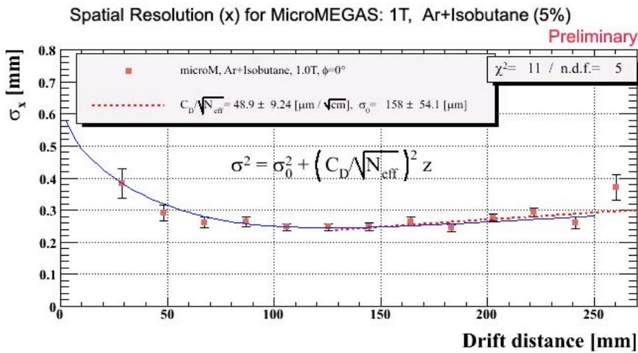
Fig. 2 Spatial resolutions measured for the MicroMEGAS in T572. The MicroMEGAS was readout by normal pads of 2.1 (2.3) mm wide (pitch) and the gas mixture was Ar-Isobutane (5%). The blue curve is the prediction from the analytic calculation with  $N_{\text{eff}}=17$ .
