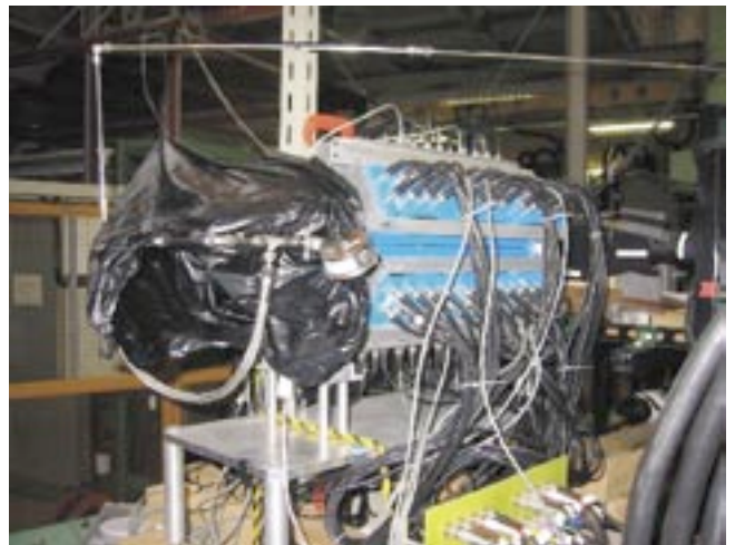
Fig. 4-2-2 Photograph of the GAPS detector with the gas target in the \pi^2 beam line.
