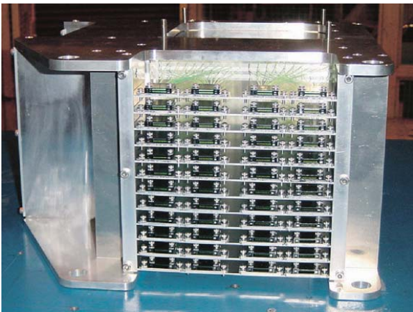
Fig. 4-2-3 R&D prototype of the electromagnetic calorimeter made of scintillator strips for experiments at the future worldwide linear colliders.
