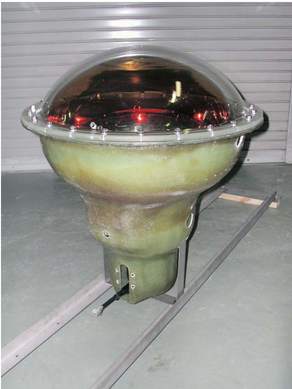
Fig. 4-3-1 An encased 20-inch PMT for the Super-Kamiokande-II detector.
