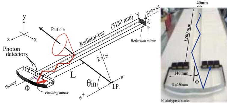
☒ 1: A schematic drawing of the TOP-counter(left) and the photograph of a prototype counter (right). The prototype has a bar of  $1,200\text{mm}^L \times 40\text{mm}^W \times 20\text{mm}^H$  size, a focusing-mirror with a curvature of  $R = 250\text{mm}$ , and 6PMTs(R5900-U-L16) as photo-detectors. Backward going photons are reflected by a mirror attached at the other bar-end and detected by the PMTs with later coming TOP than the forward going photons.
