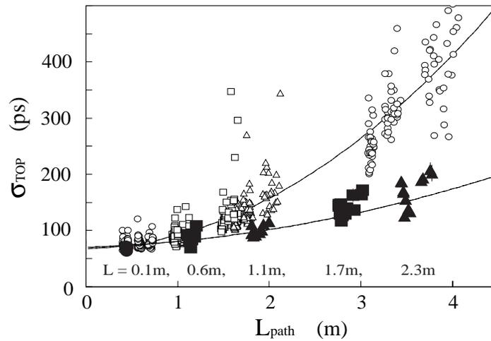
☒ 2: TOP resolution attained by the beam-tests for TOP-counter with the butterfly-shaped focusing-mirror. Open symbols are obtained by the insufficiently polished quartz-bar, while the closed ones by the newly prepared bar. Horizontal axis is the path-length along to the propagation trajectory.
