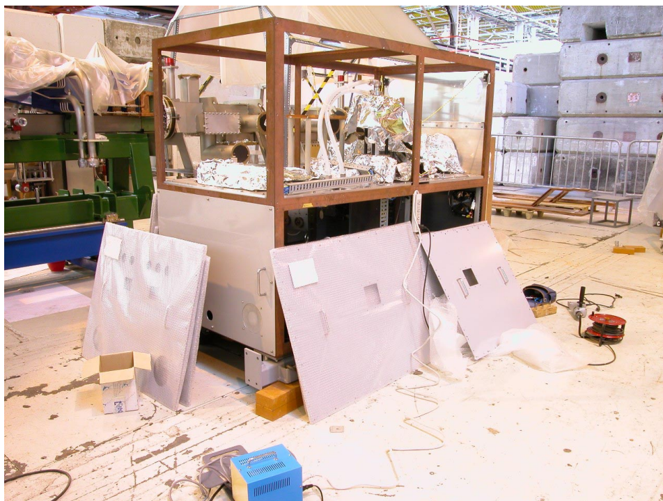
Photo 1: Work for new RF shield panels
