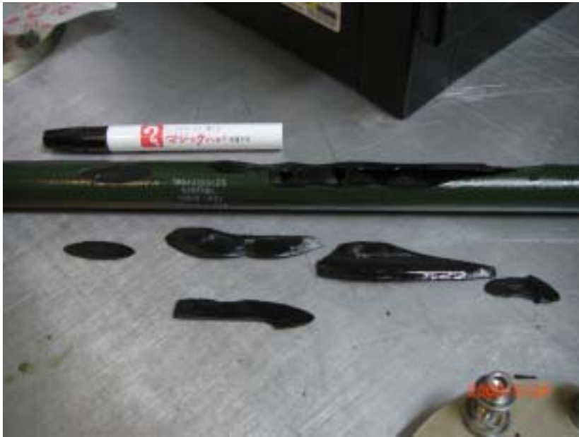
Broken damping resistor
