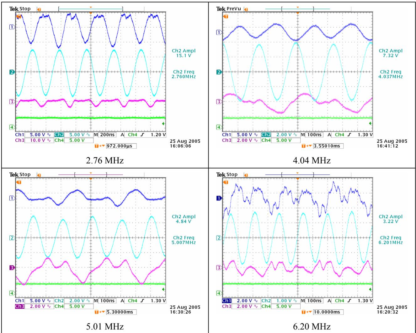
Fig.7 Waveforms in a magnified scale at 2.76, 4.04, 5.01 and 6.20MHz. From top trace, ch.1 driver stage voltage (120 $\times$ ), ch.2 cavity gap voltage (1,666 $\times$ ) ch.3 cavity input current (20A/V) and ch.4 50Hz gate pulse.
