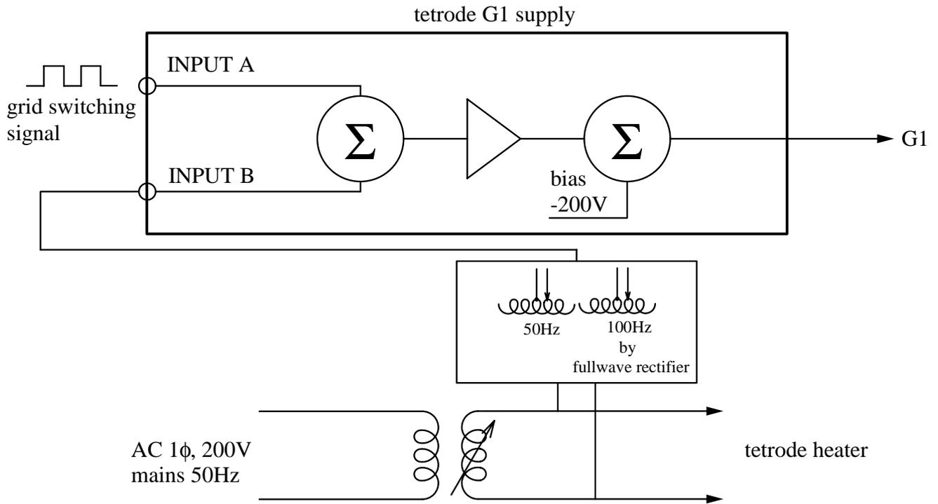
Fig.4 50/100Hz compensation for tetrode G1 supply
