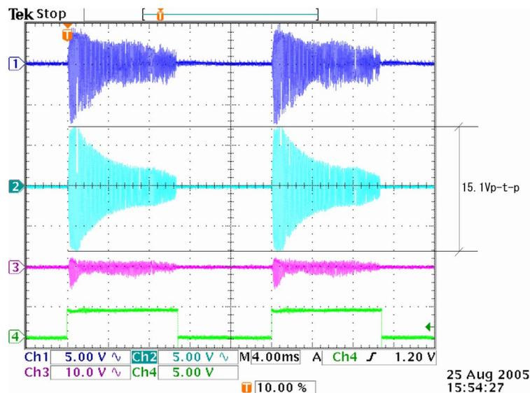
Fig.1 RF envelopes and 50Hz gate pulse. From top trace, ch.1 driver stage voltage (120 $\times$ ), ch.2 cavity gap voltage (1,666 $\times$ ), ch.3 cavity input current (20A/V) and ch.4 50Hz gate pulse. 15.1V peak-to-peak at ch.2 corresponds to 12.6KV peak per gap.
