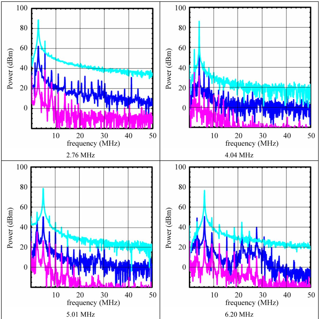
Fig.9 FFT results of the waveforms in fig.7 in the frequency range of 0~50MHz. From top trace, cavity gap voltage (light blue), driver stage voltage (blue) and cavity input current (red).
