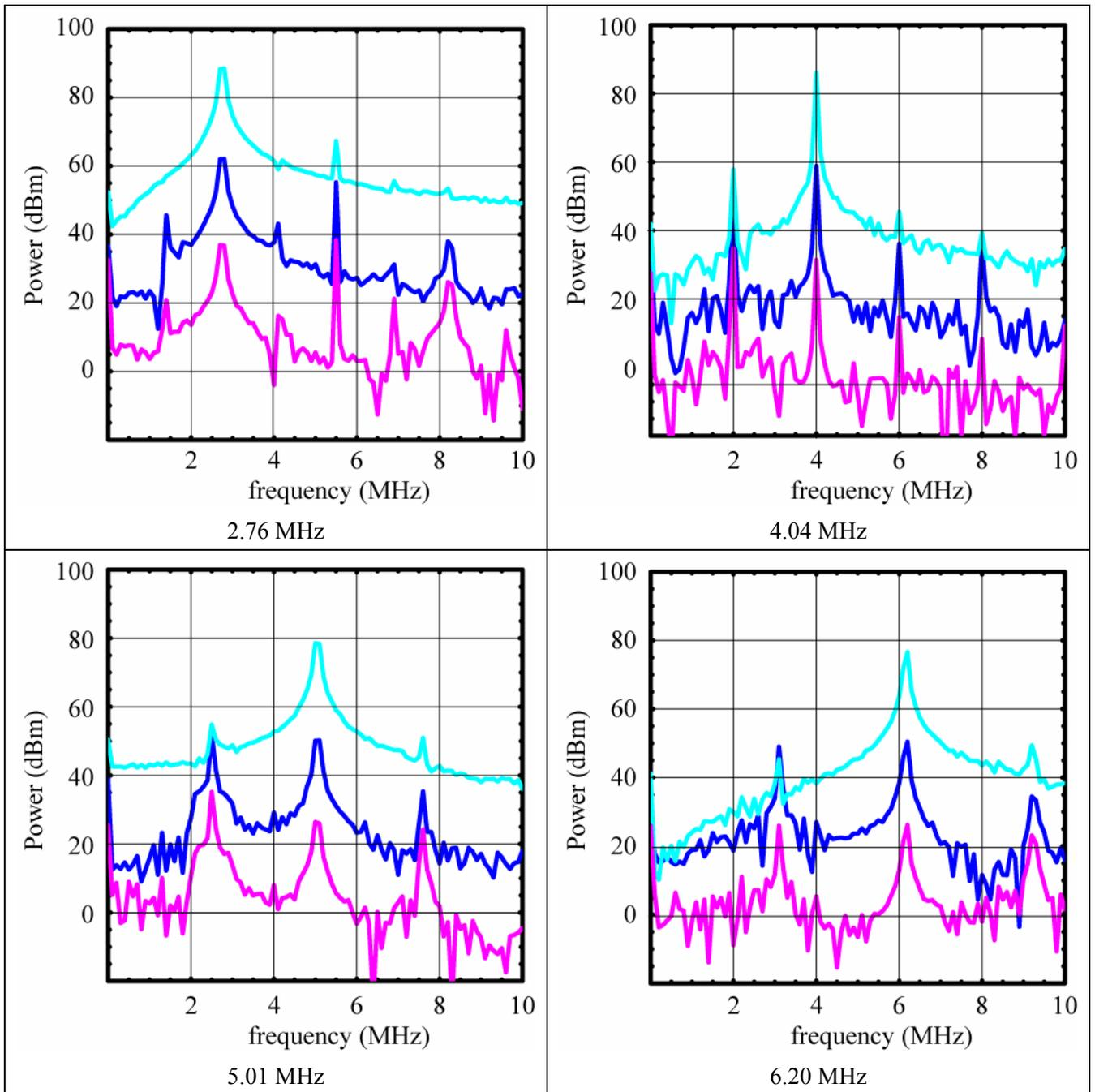
Fig.8 FFT results of the waveforms in fig.7 in the frequency range of 0~10MHz. From top trace, cavity gap voltage (light blue), driver stage voltage (blue) and cavity input current (red).
