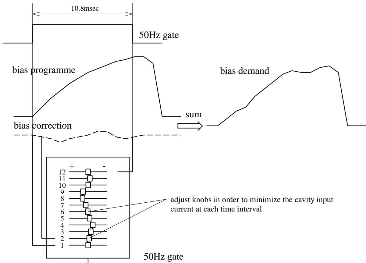
Fig.5 Cavity bias correction
