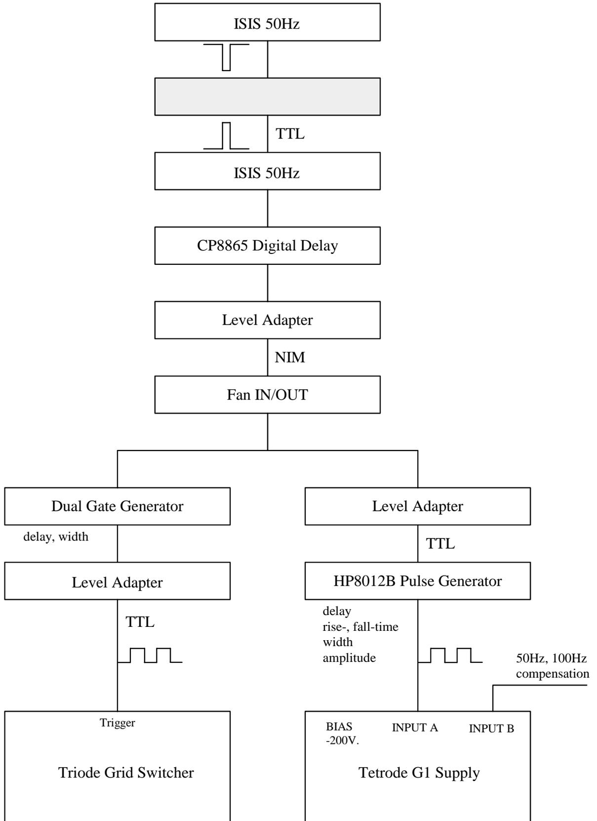
Fig.3 Grid switching schematic
