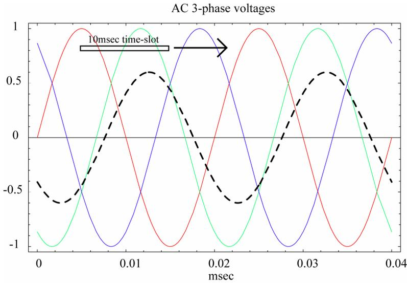
Fig.6 3 $\phi$  voltage input (solid) of the tetrode supply and 50Hz pattern (dotted) showing some vibrations of the heater filament synchronizing with one of the three phases. Time slot with 10msec duration moves at a beat frequency.
