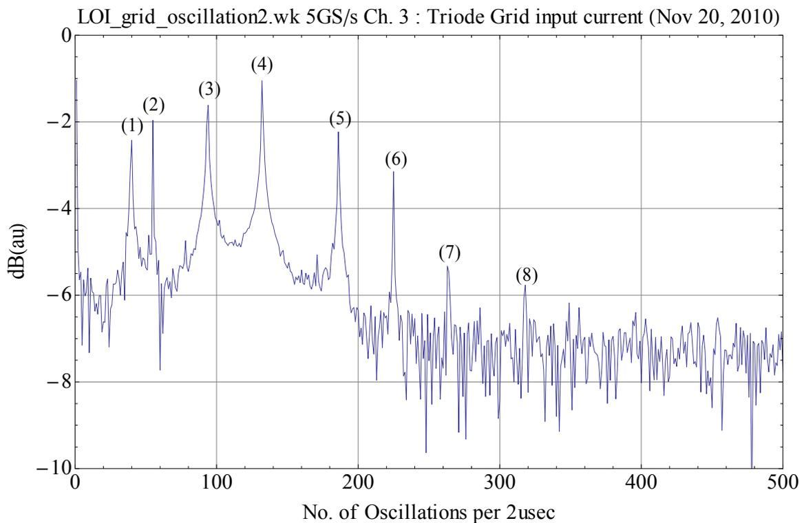
FFT: (1) 20.0MHz, (2) 27.4MHz, (3) 46.8MHz, (4) 66.1MHz, (5) 93.2MHz, (6) 112.5MHz, (7) 131.9MHz, (8) 159.0MHz.
