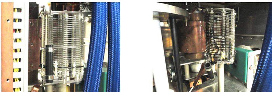
Fig. 3 New feedback coil before RF on (left), which was burnt after RF test in November 20, 2010 (right).
