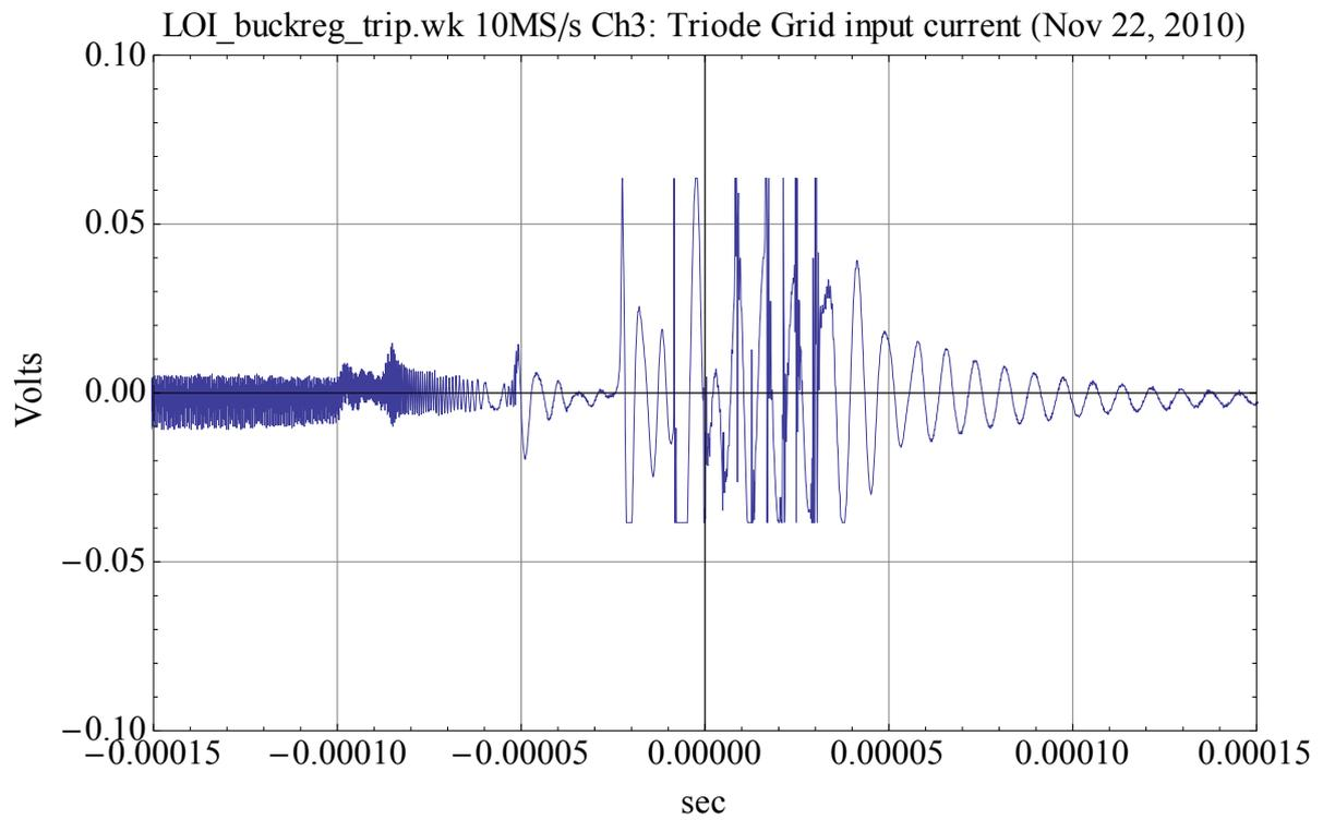
Ringling frequency:  $\sim 3.3\text{MHz}$  (left part) and  $158 \sim 127\text{kHz}$ (right part).
