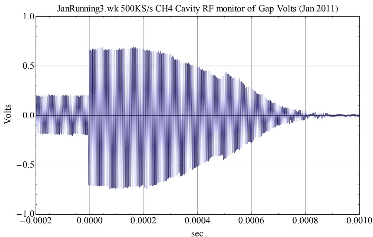
Step-function increase at 0sec ( $\times 3.5$ ). **This increase does not correspond to that of grid volts!!**
