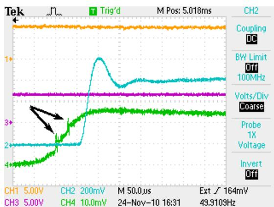
Fig. 10 From top trace, BR output voltage, tetrode supply output voltage, BR output current and tetrode supply output current. Tetrode current spikes are shown with arrows.
