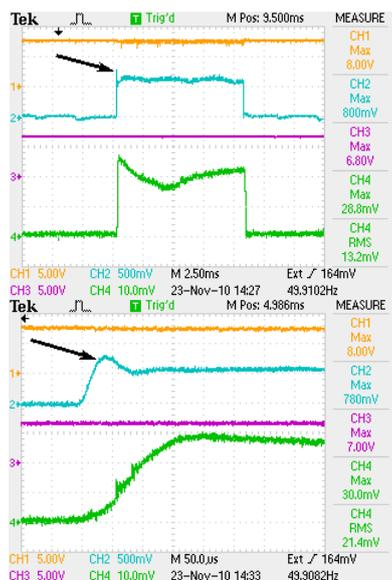
Fig. 8 From top trace, BR output voltage and current, tetrode supply output voltage and current after the RF test in November 20, 2010. Overshoot is shown with an arrow at the BR output current.
