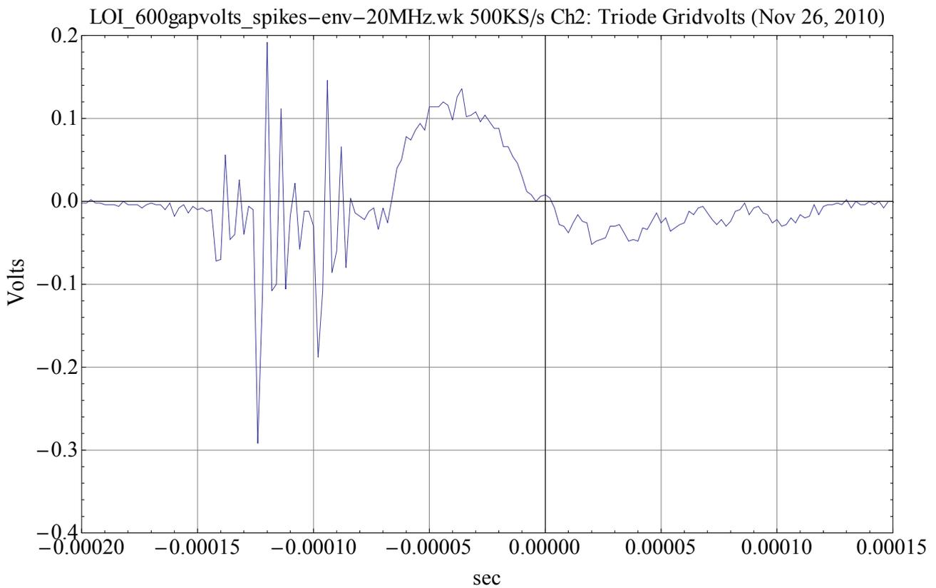
At the beginning of anode switching: ringing frequency is 170kHz, width of broad peak is ~70usec.
