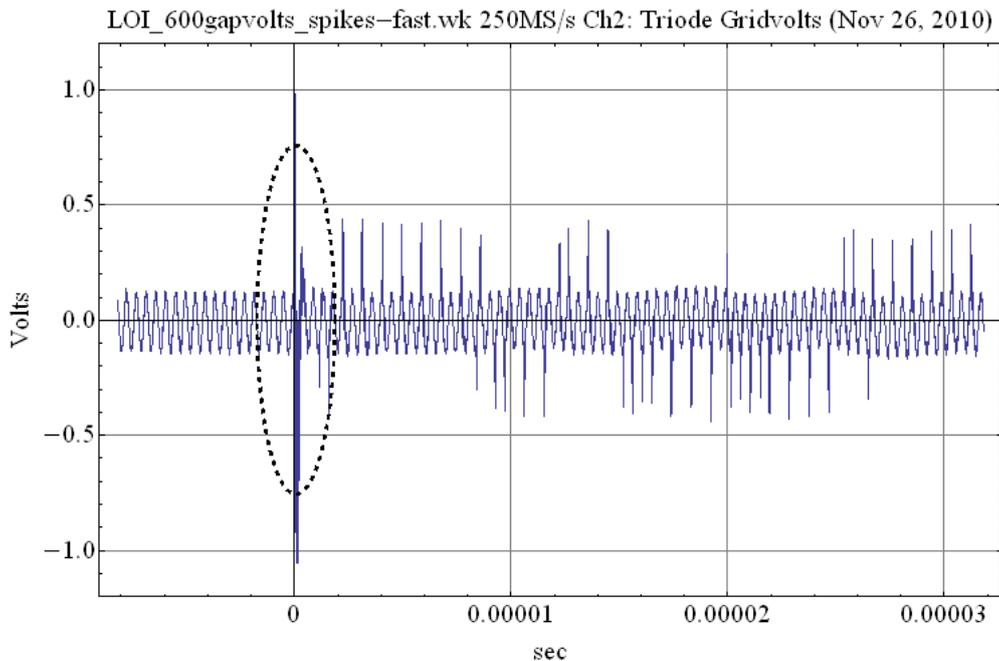
Frequency of the continuous wave is 2.207MHz.
