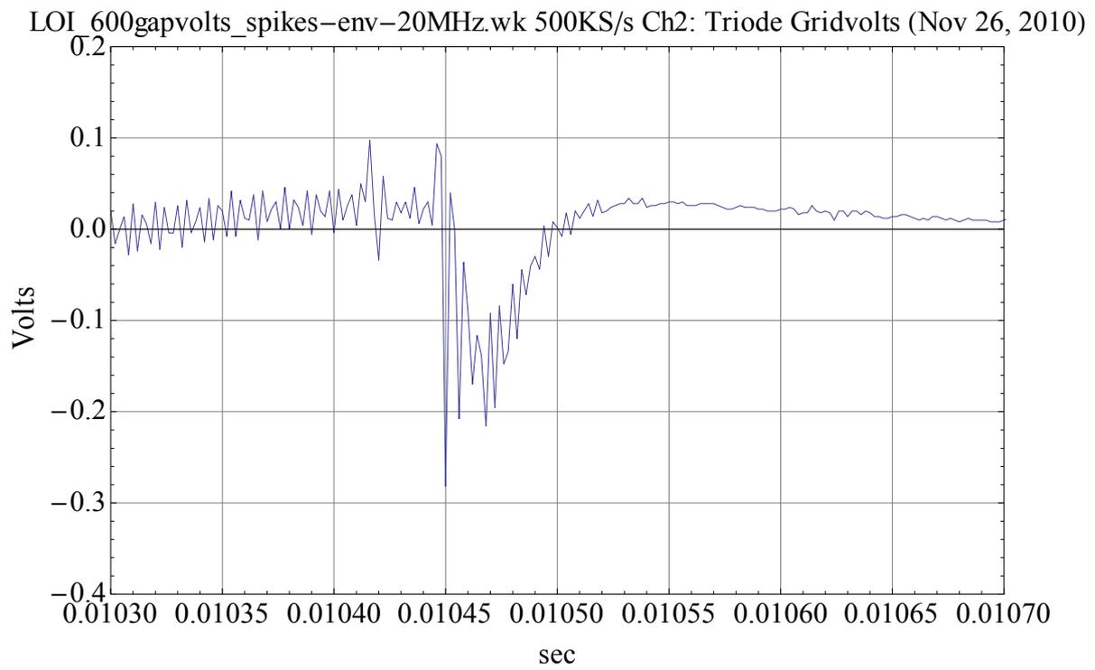
At the end of anode switching: ringing frequency is 100.0kHz, width of broad peak is ~50usec.
