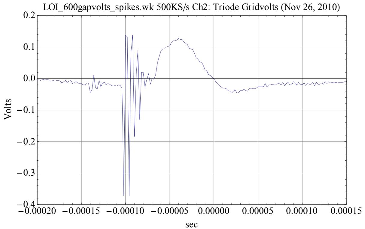
Triode gridvolts at the beginning of anode switching: ringing frequency is 156kHz, width of broad peak is ~80usec.
