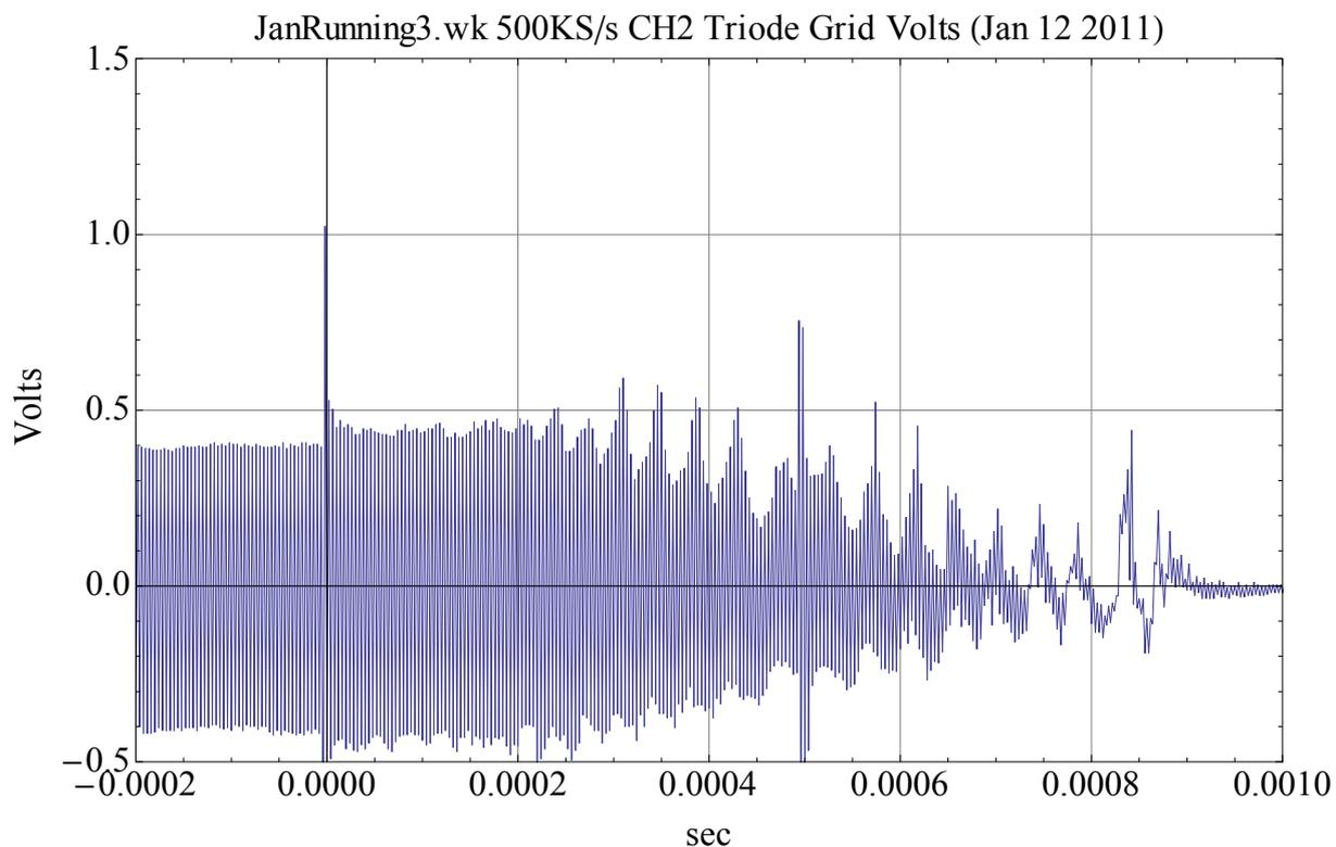
Large spike ( $\times 2.5$ ) at 0sec, followed by a bit larger amplitude ( $\times 1.1$ ) with 25.4kHz modulation.
