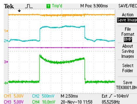
Fig. 9 From top trace, BR output voltage and current, tetrode supply output voltage and current before the RF test in November 20, 2010.
