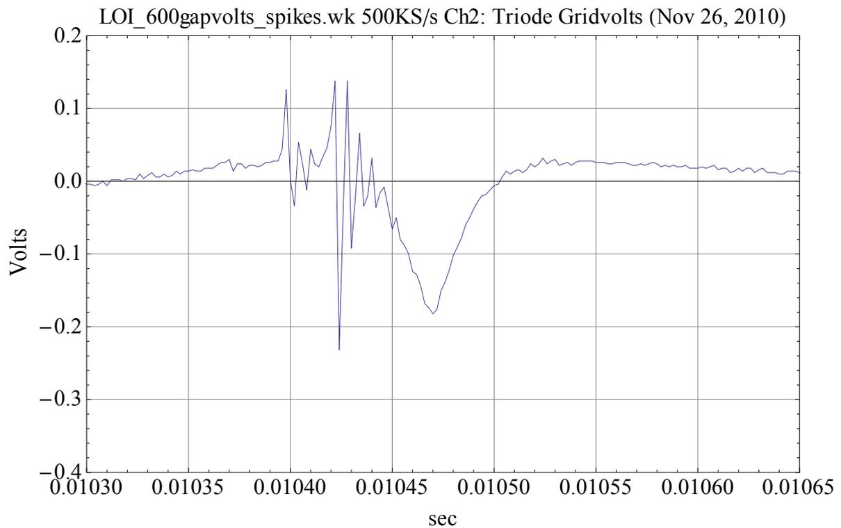
Triode gridvolts at the end of anode switching: ringing frequency is 167kHz, width of broad peak is ~60usec.
