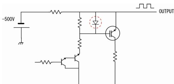
Fig. 6 Proposed surge absorber to the grid switcher in the dotted circle.
