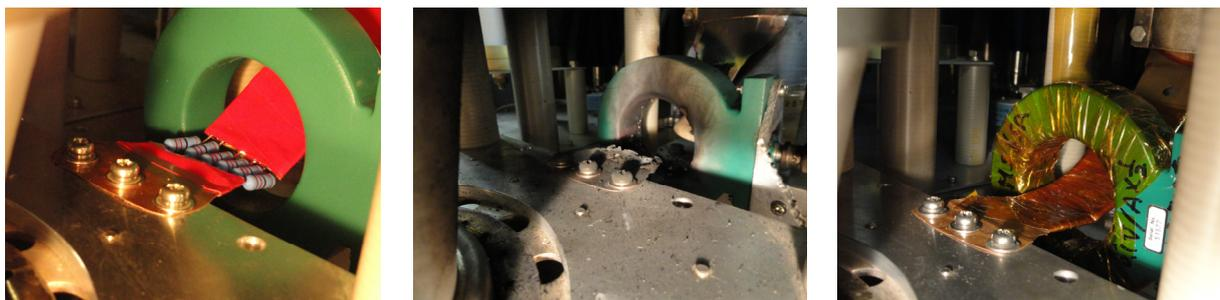
Fig. 13: Grid input resistor before burning (left) and after (middle). Grid input circuitry was repaired without grid input resistor and using a used current transformer, Pearson model 110 (right).
