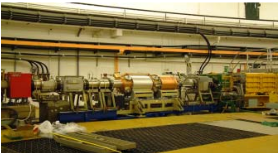
SP6 cavity installed and vacuum restored.
