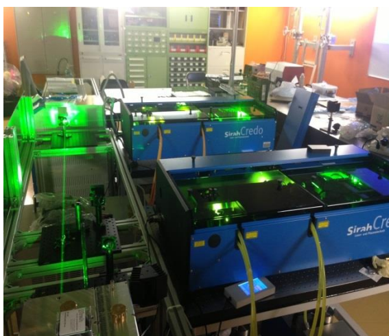
Figure 9. The photograph of new PALIS lasers: shining two dye lasers pumped by YAG laser.
