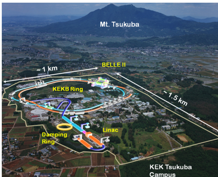
FIG. 1. (Color online) Schematic layout of the SuperKEKB in the KEK Tsukuba campus.
