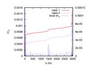
Figure 3: Vertical tune shift along the ring.
