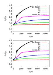
Figure 8: Evolution of the vertical beam size for various electron density. Top and bottom pictures depict the evolutions for the cases (1) and (2).
