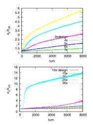
Figure 6: Evolution of the vertical beam size for various electron cloud density. In the top picture, electrons distribute only IR, s < 75 and s > 2940 m. In the bottom picture, electron distribute only in arc section, 75 < s < 2940 m. The electron cloud distribution is the case (1).
