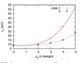
Figure 9: Equilibrium emittance as functions of the electron cloud density. Two lines, red and blue, are drawn for the cases (1) and (2), respectively.
