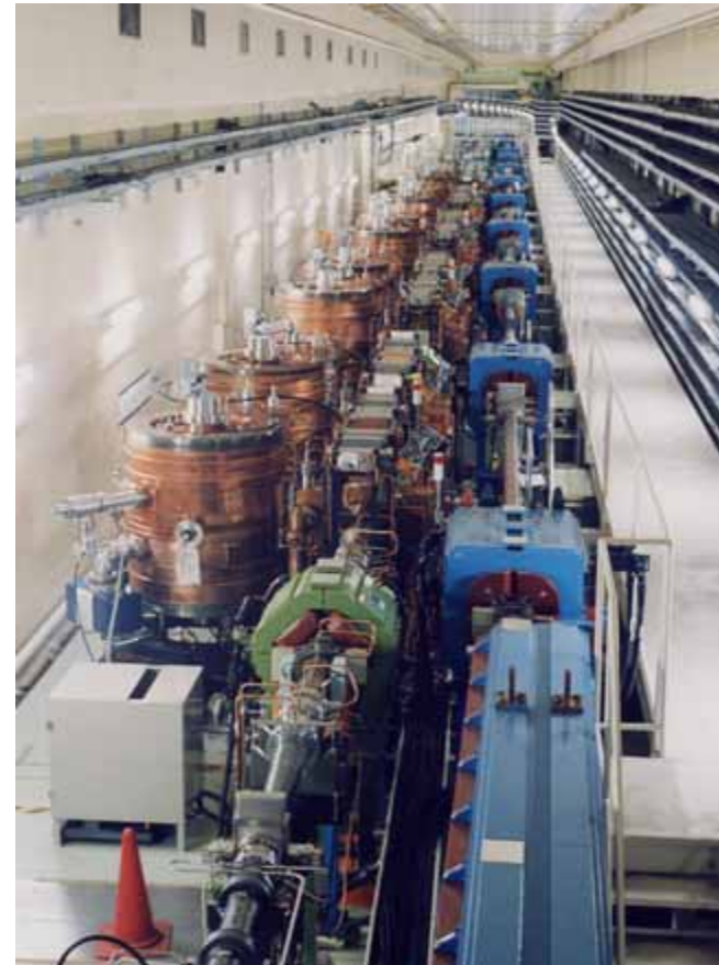
ARES cavities in the LER RF section
