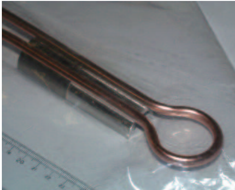
Figure 2: The test piece with a cooling copper tube brazed on the outer surface.
