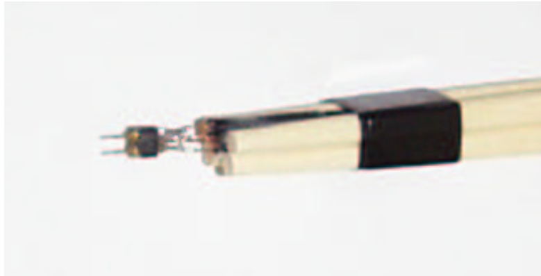
Figure 7: The Au-coated pin head used as a probe in the resistance measurement. Two lead wires are connected to each pin for the four-wire measurement.
