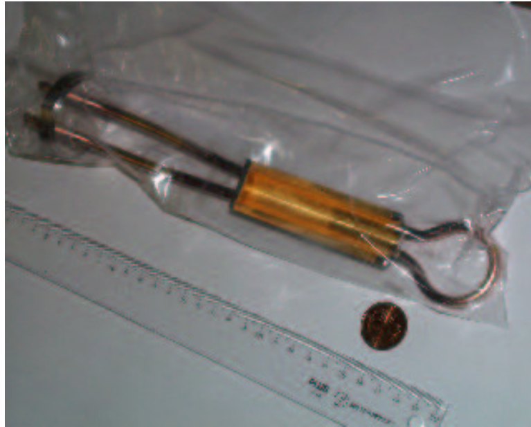
Figure 3: The test piece with an Au coating on the inner surface.
