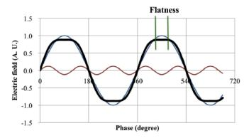
Figure 10: RF field flatness formation by superimposing with the 3<sup>rd</sup> harmonic RF with 12% of main RF field.
