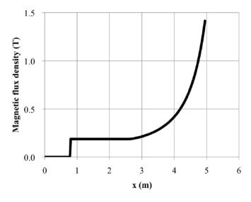
Figure 6: Variation of magnetic flux density, satisfying the isochronous condition (solid line) in the case of the recirculating LINAC.
