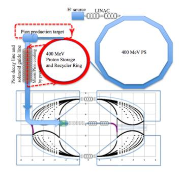
**Figure 13:** Overview of the entire accelerator complex for muons. In the case of the multi-purpose proton driver such as cyclotron or synchrotron, the proton storage ring or recycler ring is required to wait low-repetition rate pulse systems for high-field devices ready. The scale unit of grids is [m].
