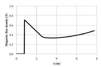
**Figure 20:** Variation of magnetic flux density, satisfying the isochronous condition for 40 MeV protons accelerated up to the energy of 400 MeV.
