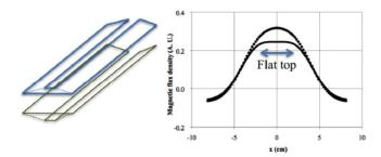
**Figure 19:** Overview of the kicker magnet excited by a fourturn coil (left). Horizontal uniformity is obtained by using the coil-winding method (the solid line in the right panel). Curved lines (dotted lines) are obtained in almost all cases describing the variation of the magnetic flux density excited by the simple flat four-turn coil.
