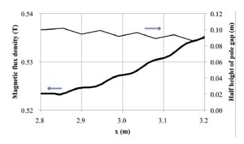
Figure 11: Magnetic field modulation (solid line) by step pole surface (thin line) in the main magnets for simulated synchrotron oscillation.
