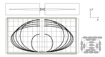
Figure 5: Representative muon trajectories for the recirculating LINAC, compared with simple LINAC (bottom panel) and spiral LINAC (right panel) sizes. Top panel shows the cross-section of main magnets. The scale unit of grids is [m].
