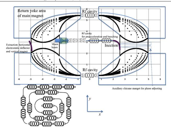
**Figure 7:** Representative muon trajectories for the racetrack FFAG, compared with spiral LINAC size. The scale unit of grids is [m].
