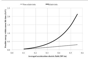
**Figure1:** Muon energy (during its lifetime) versus averaged accelerating electric field. The thin and the solids indicate calculation results for non-relativistic and relativistic estimations, respectively. Electric field intensity of 0.28 MV/m is required for accelerating muons to the energy of 300 MeV.
