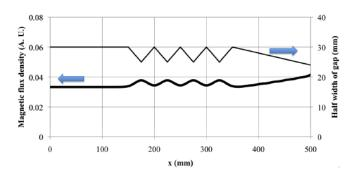
Figure 9: Magnetic field modulation. The sawtooth pole surface, marked by the thin line, can yield field modulation, as the solid line indicates.
