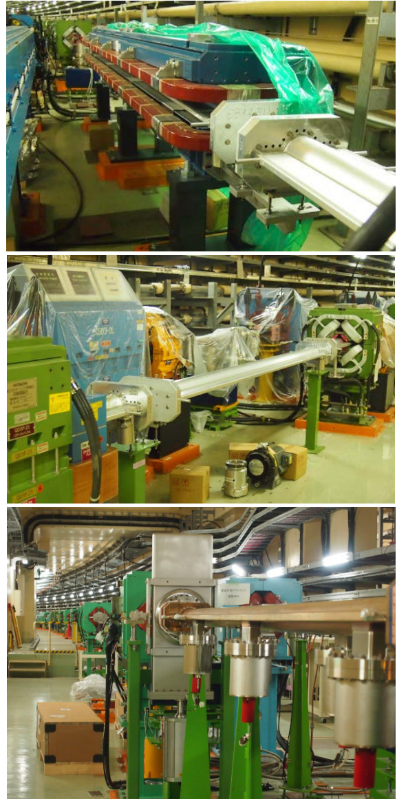
Figure 5: Beam pipes for bending magnets and for drift spaces, and gate valves installed in the LER arc section for test.
