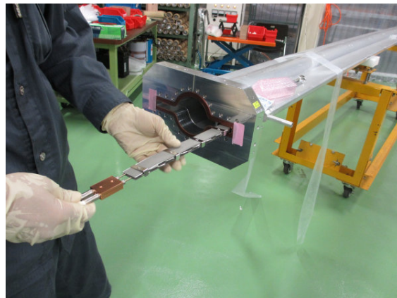
Figure 3: NEG pumps (NEG strips and micro-heaters for activation) integrated in a beam pipe with antechambers.
