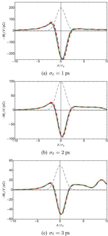
Figure 2: CSR wake potentials for a single bend in the cERL return loop with Gaussian bunch lengths of  $\sigma_t = 1, 2, 3$  ps. The drift CSR is taken into account. Blue solid lines:  $\gamma=\infty$ ; red dashed lines:  $\gamma=68.5$  ( $E=35$  MeV); green dashed lines:  $\gamma=244.6$  ( $E=125$  MeV); gray dashed lines: Gaussian bunch profile.
