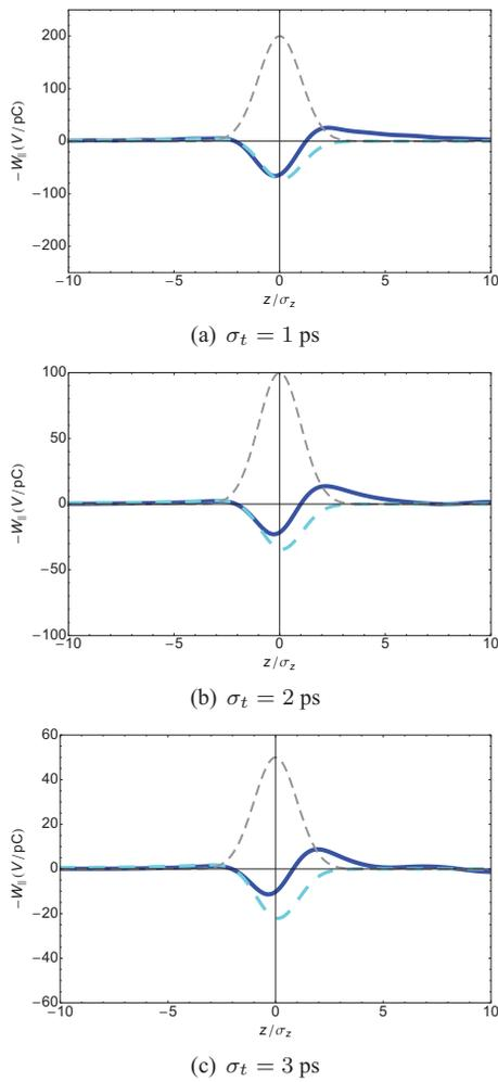
Figure 6: CSR wake potentials for a single bend in the cERL return loop with Gaussian bunch lengths of  $\sigma_t = 1, 2, 3$  ps and  $\gamma = \infty$ . Blue solidlines: drift CSR by CSRZ; cyan dashed lines: drift CSR by Stupakov and Emma's free-space model; gray dashed lines: Gaussian bunch profile.
