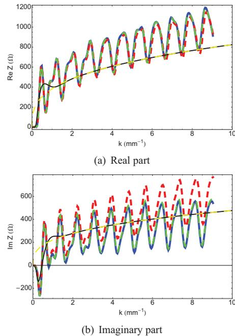
Figure 1: CSR impedance for a single bend in the cERL return loop. The CSR in the drift chamber after the exit of the bend is taken into account. Blue solid lines:  $\gamma = \infty$ ; red dashed lines:  $\gamma = 68.5$  ( $E = 35$  MeV); green dashed lines:  $\gamma = 244.6$  ( $E = 125$  MeV); black solid lines: steady-state parallel plates model; yellow dashed lines: steady-state free space model.
