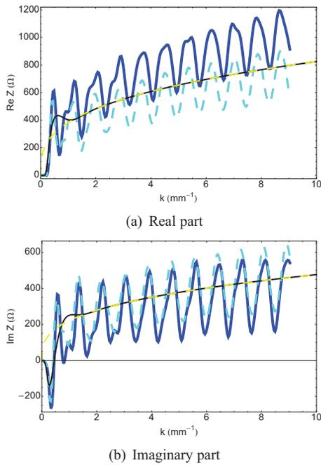
Figure 4: CSR impedance for a single bend in the cERL return loop with  $\gamma = \infty$ . Blue solid lines: with drift CSR considered; cyan dashed lines: with drift CSR neglected; black solid lines: steady-state parallel plates model; yellow dashed lines: steady-state free space model.
