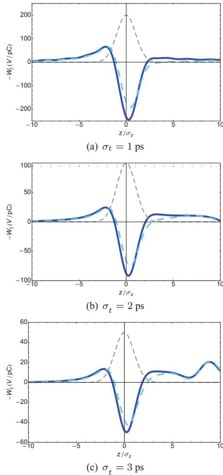
Figure 5: CSR wake potentials for a single bend in the cERL return loop with Gaussian bunch lengths of  $\sigma_t = 1, 2, 3$  ps and  $\gamma = \infty$ . Blue solidlines: with drift CSR considered; cyan dashed lines: with drift CSR neglected; gray dashed lines: Gaussian bunch profile.
