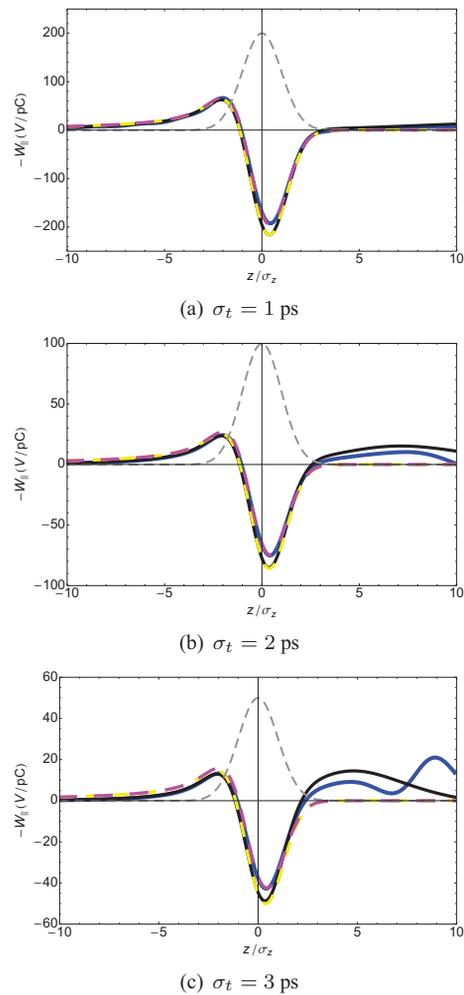
Figure 3: CSR wake potentials for a single bend in the cERL return loop with Gaussian bunch lengths of  $\sigma_t = 1, 2, 3$  ps and  $\gamma = \infty$ . The drift CSR is not taken into account. Blue solid lines: by CSRZ; magenta dashed lines: 1D model; black solid lines: steady-state parallel plates model; yellow dashed lines: steady-state free space model; gray dashed lines: Gaussian bunch profile.
