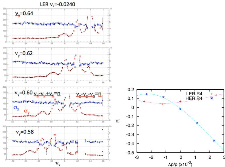
Figure 8: Measurement of the beam size in tune space and of chromaticity for R4 (by Y. Ohnishi & K. Ohmi).
