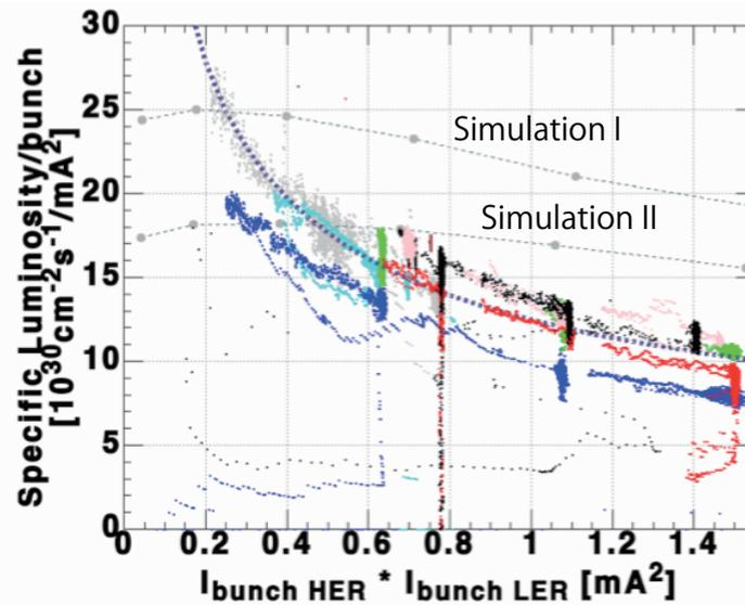
Figure 3: Specific luminosity as function of current product of two beams.
