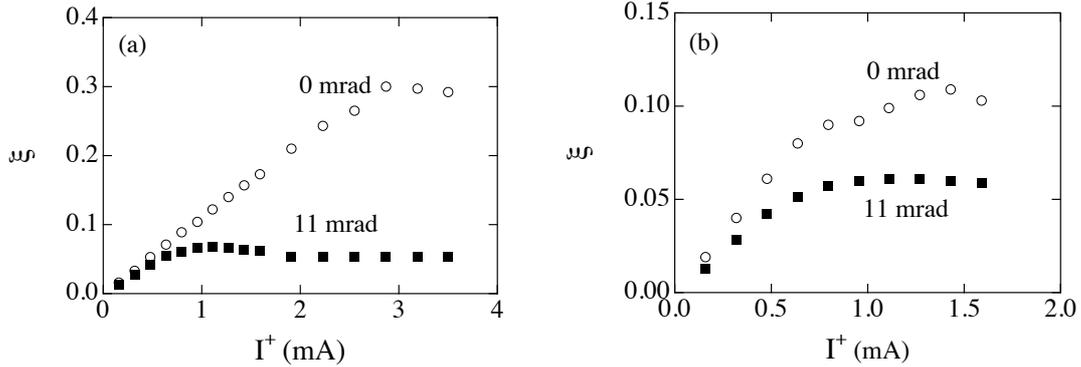
Figure 1 Beam-beam parameter as functions of positron current. Electron current is changed with the same ratio. Plots (a) and (b) are obtained by beam-beam simulation codes with the weak-strong (BBWS) and strong-strong (BBSS) model, respectively.
