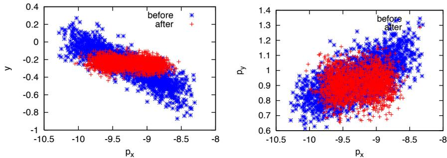
Figure 5: Phase space at IP measured by nearby turn by turn monitors (OctoPos).
