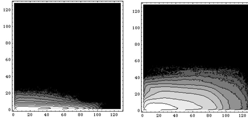
Figure 10: Beam distribution in the transverse space with (left) and without (right) crab cavity given the beam-beam simulation (BBWS). The full scale of the pictures is 0-12.8  $\sigma_x$ , 0-64  $\sigma_y$  for horizontal and vertical, respectively.
