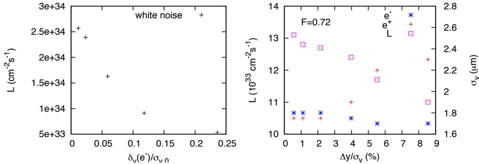
Figure 9: Luminosity for the vertical beam fluctuation amplitude. Left and right plots are given for the simulation and measurement (by M. Tobiyama & K. Ohmi).
