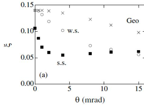
Figure 2: Beam-beam parameter for crossing angle. Three kinds of dots are given by geometrical luminosity (Geo) and simulated luminosity using weak-strong (w.s) and strong-strong (s.s) model.
