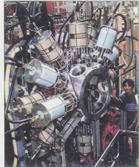
Squeeze play. Gamma rays entering the 14 spokelike detectors of Tohoku University's Hyperball instrument showed evidence of pint-sized lithium nuclei.
