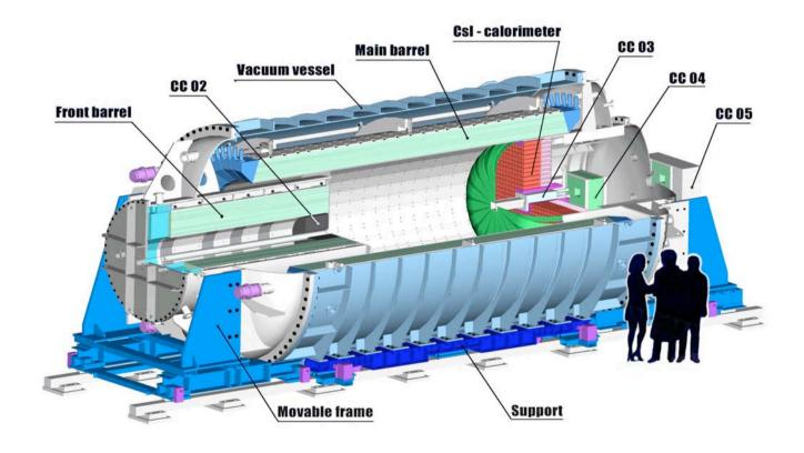
100-ton calorimeters are installed in vacuum chamber
