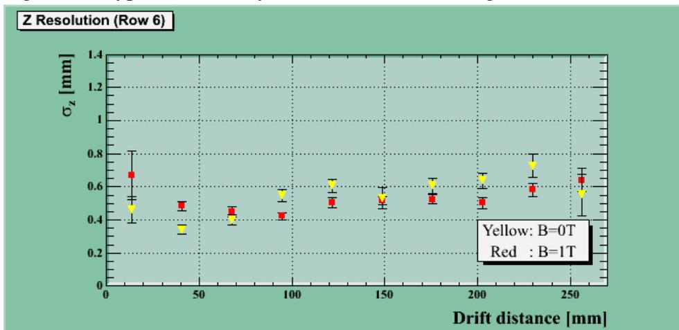
Fig.3. Point resolution measured as a function of drift distance in MWPC-TPC (preliminary)
