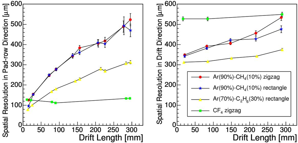
Figure 1: Spatial resolution of the TPC versus the drift length in the pad-row direction (left) and the drift direction (right).
