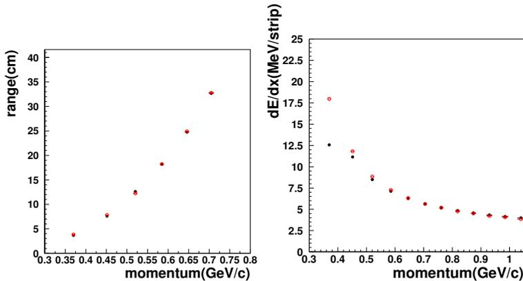
Figure 1: Measured range (left) and  $dE/dx$  (right) of protons in scintillator as a function of momentum. Black (red) points represent data (MC).
