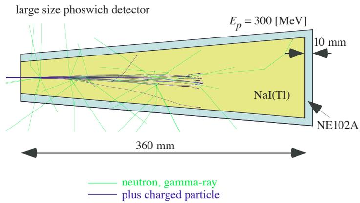
Fig. 1 Schematic of the phoswich type recoil proton detector
