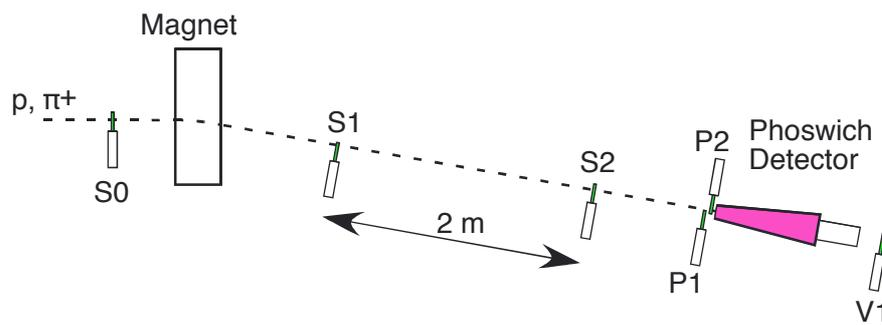
Fig. 2 Detector arrangement at  $\pi^2$  beam line
