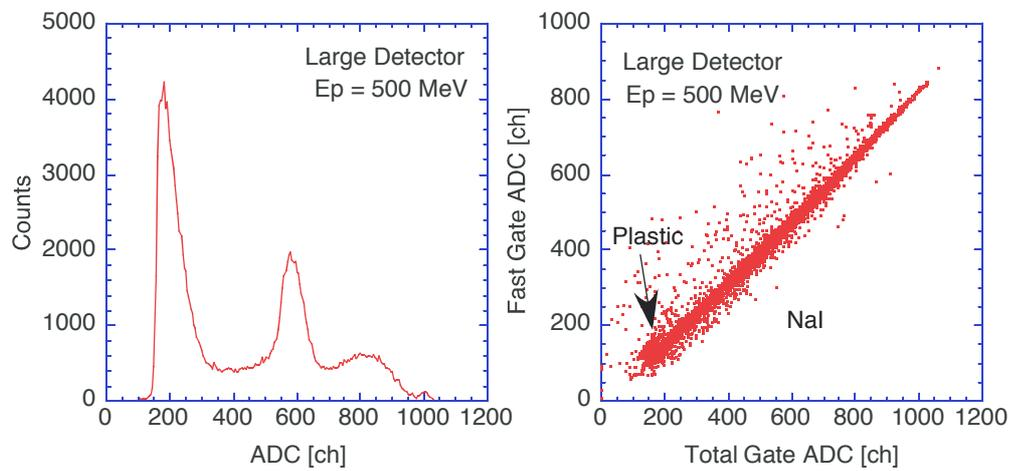
Fig. 3 ADC spectrum and pulse shape discrimination of the phoswich detector
