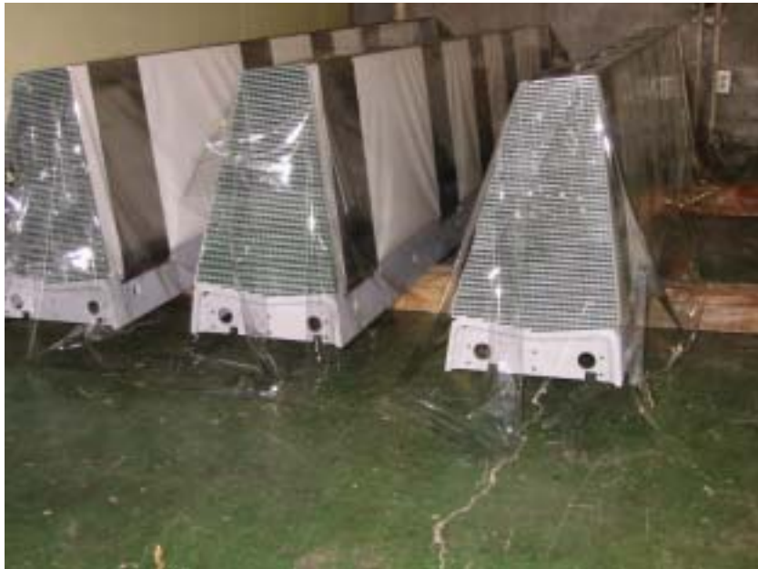
Fig. 4. Fabricated modules of the front barrel. Total number of modules is 16 and they will be assembled into the front barrel veto.
